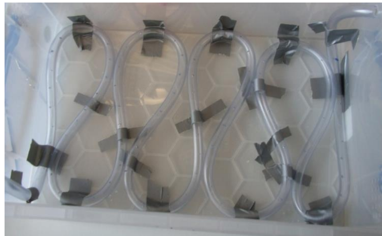
Figure 2.6: Photo of hypoxia box showing holed plastic tubing through which CO 2 enters the box.
