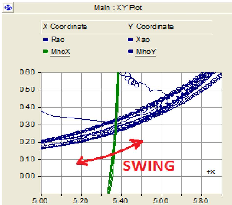
Figure 5.21: The impedance swing in and out of the DR zone
