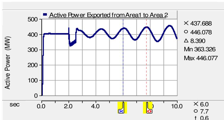
Figure 4.7: Inter-area mode of oscillation
