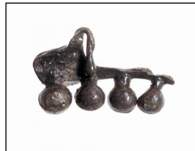
Figure 5.25. Lead shot still attached to casting runner (Preservation Virginia).
