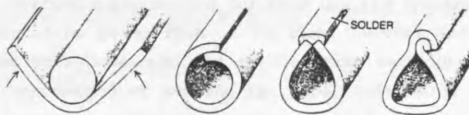
c) forming pipe and showing soldered and lap joints
