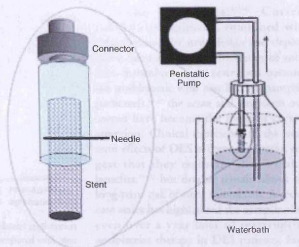
**Figure 2.** *In vitro* perfusion circuit for elution of eptifibatide from polymer-coated stents. The standard flow rate used was 25 ml min<sup>-1</sup>. In the platelet deposition experiments, the PBS was replaced by blood containing 111Indium labeled platelets.
