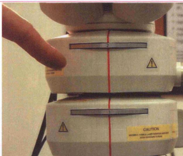
Fig. 3.4. Position of the switching mechanism below trinocular head.
