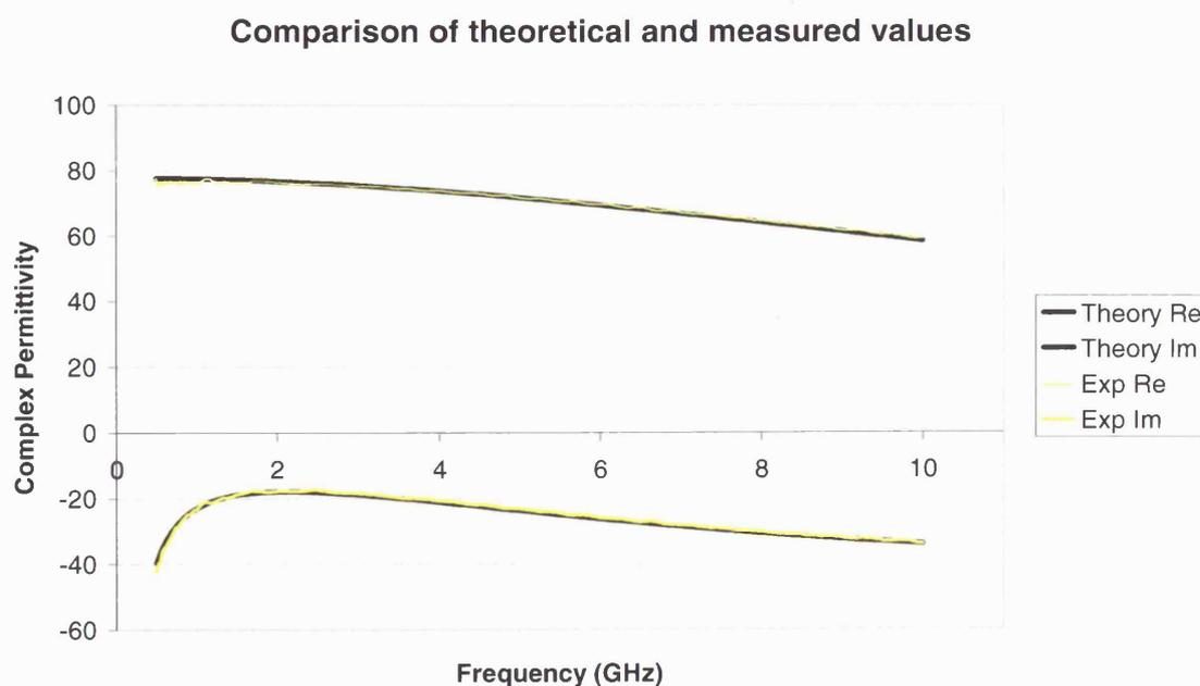
**Figure. 6.** Agreement between measured and theoretical complex permittivity over microwave frequencies of 0.5-10 Gigahertz of 0.1% saline solution.
