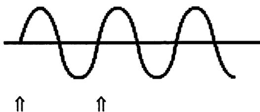
**Figure 2.1.** Typical graphic of a wave, the distance between the two arrowheads depict 1 wavelength ( $\lambda$ )
