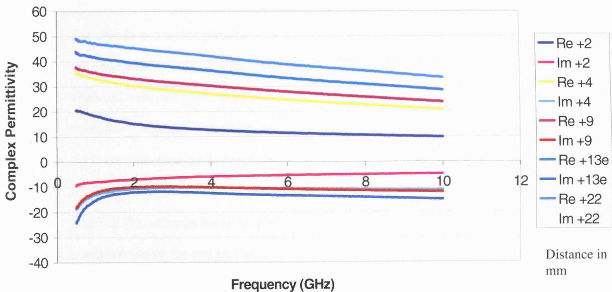
**Figure 5.** Shows the real and imaginary readings taken after a 120 second microwave treatment in porcine liver at a power of 150 Watts at increasing intervals from the burn epicentre. Re +2 indicates the real portion of permittivity at a distance of 2mm from the burn epicentre, Im +2 represents the imaginary portion of complex permittivity reading obtained at a distance of 2mm from the burn epicentre. Other figures following the Re (real) or Im (Imaginary) designate the distance from the burn
