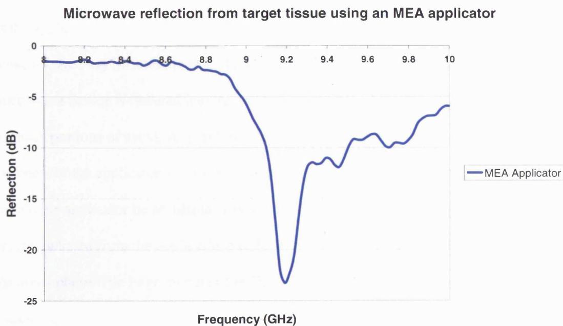
**Figure 2.9.** Reflection of microwaves from the applicator/endometrium interface.
