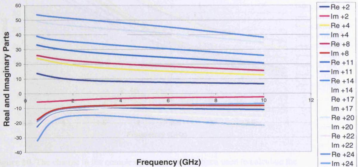
**Figure 9.** The change in complex permittivity in a human colorectal metastasis following a microwave ablation treatment of 300 seconds at 150 Watts. This graph should be interpreted along the lines of Figure 5. The results show very similar results to those in Figure 5 in that both the real and imaginary portions of complex permittivity have been affected by the treatment in a manner that is that proportional to the distance from the applicator.
