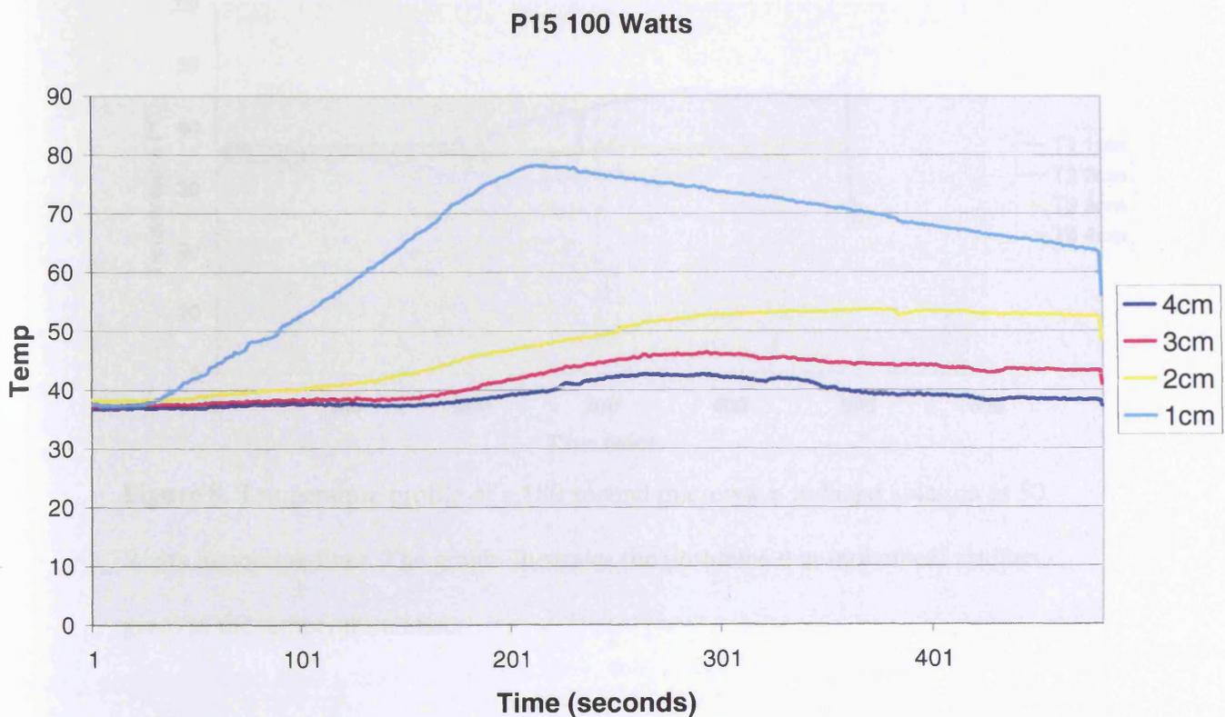
**Figure 7.** Temperature readings obtained from the thermocouples mounted within the aluminium jig during a 100 Watt ablation. This was a good, smooth trace although many of the traces obtained from the ablations were not of the quality of this.
