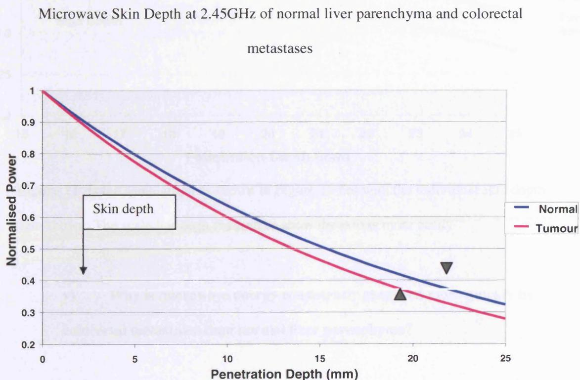
**Figure 10.** Microwave Skin Depth in human liver parenchyma and hepatic colorectal metastases. The X axis is in millimetres and the Y axis is a fraction of the energy of the wave. The white line is the mathematically defined point at which skin depth is calculated (i.e. the distance that the wave has to pass through the tissue to lose 67% of its original energy). The two arrowheads indicate the increased skin depth in normal liver parenchyma when compared to that of the tumour tissue (2.5mm).
