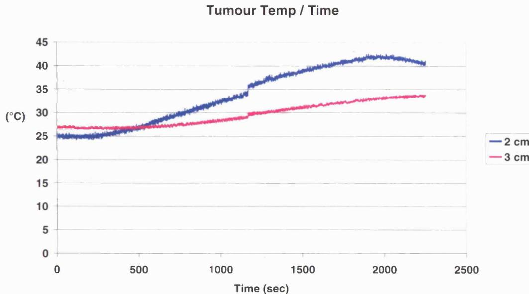
**Figure 1.** Increase in temperature at 2 and 3 cm intervals from the microwave applicator following treatment of ex-vivo liver with a 9.2GHz microwave applicator using 30 Watts.
