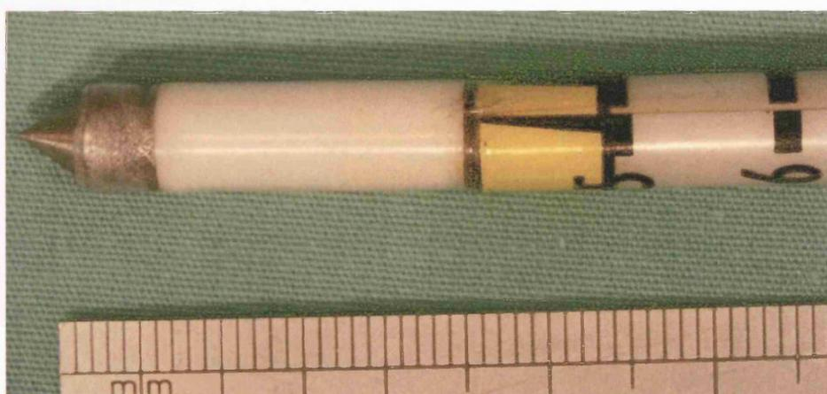
**Figure 2.15.** Close up of the radiating portion of the 2.45GHz interstitial microwave applicator.
