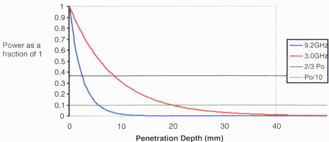
**Figure 2.** Skin depth (black line  $2/3 P_o$  where  $P_o$  is the initial or incident power i.e. the point at which the wave has lost approximately 2/3 of its power or amplitude known as the skin depth) calculation for normal liver at 9.2 and 3.0 GHz. It is
