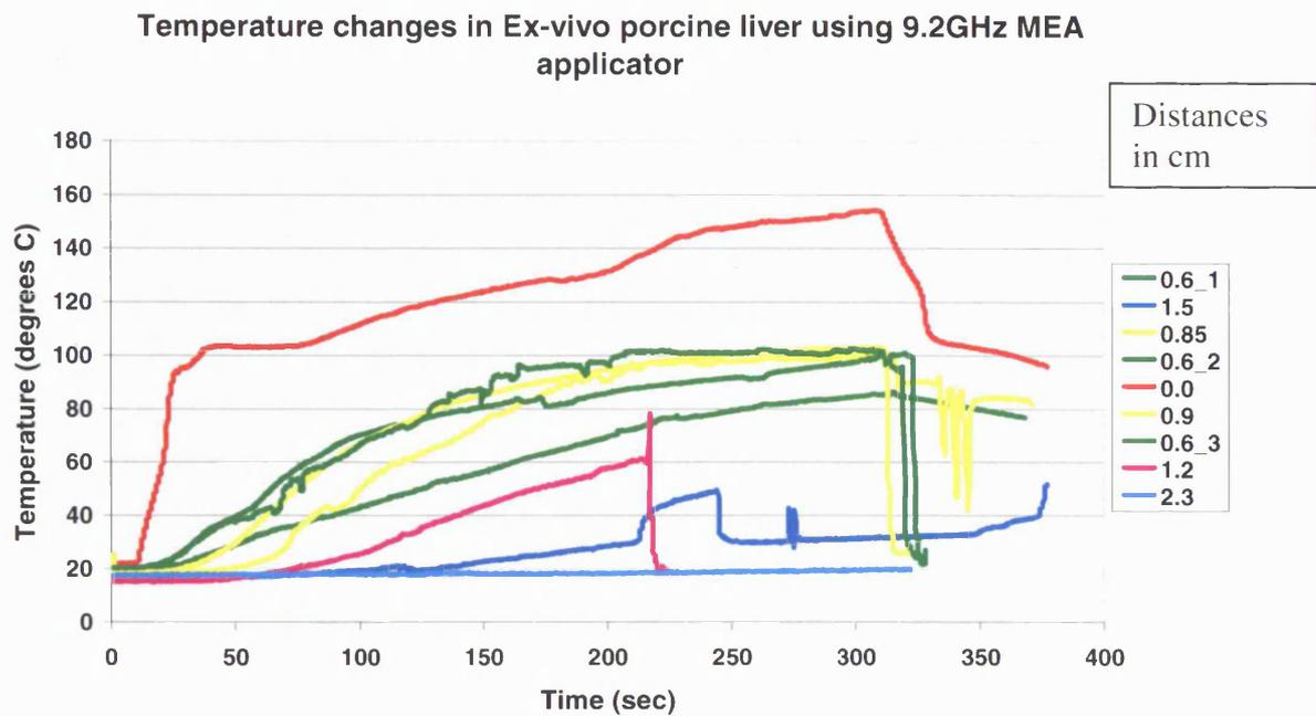
**Figure 2.** Increase in temperature at different intervals from the applicator (in cm) as measured by metallic thermocouples. The steep gradient (representing rapid heating) of the red line at 0cm from the applicator is of interest as this illustrates the effect of direct field heating on the thermocouple.
