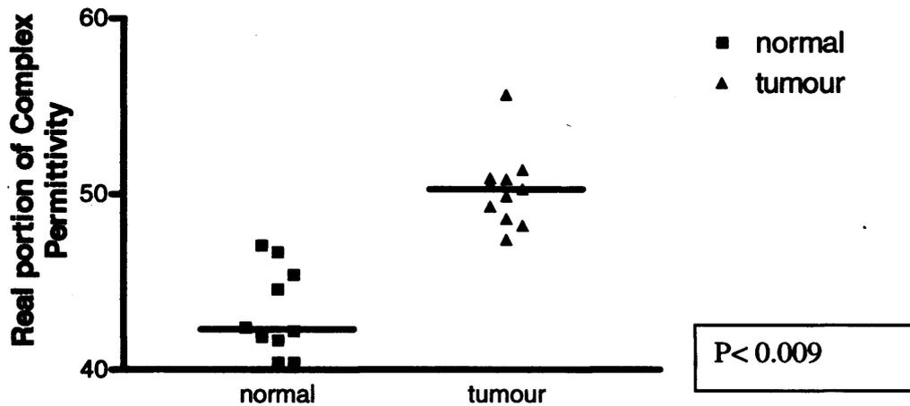
**Figure 8.** Real portion of complex permittivity at the microwave frequency of 2.45GHz. A highly significant difference is seen between the two tissue types at this microwave frequency indicating tumour tissue takes/stores more microwave energy than normal liver parenchyma.
