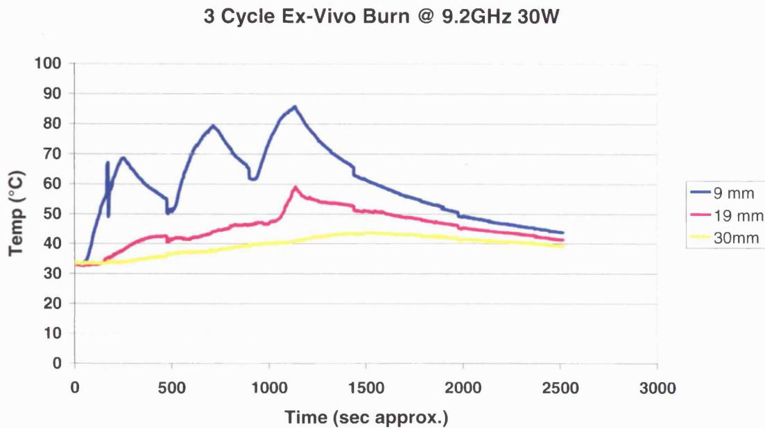
**Figure 3.** Temperature profiles of thermocouples placed at 9, 19 and 30 millimetres.
