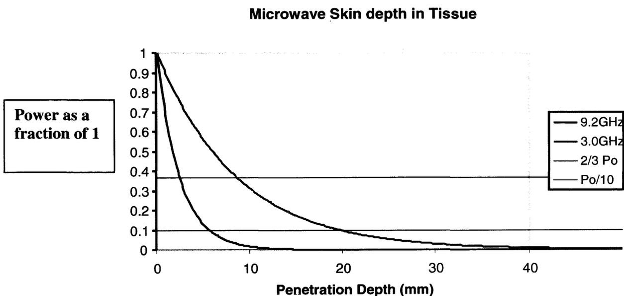
**Figure 2.7.** Graph showing the effect of frequency on penetration of microwaves through tissue. Microwave penetration through tissue is known as skin depth and is defined by the distance at which approximately  $2/3$  of the incident power has been dissipated (black line).
