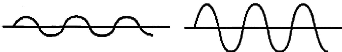
**Figure 2.2.** Comparison between two waves of equal wavelength but different amplitudes. The wave to the right of the figure shows far more deviation from the mean (line drawn through the middle of each waveform) indicating it carries a greater amount of energy.
