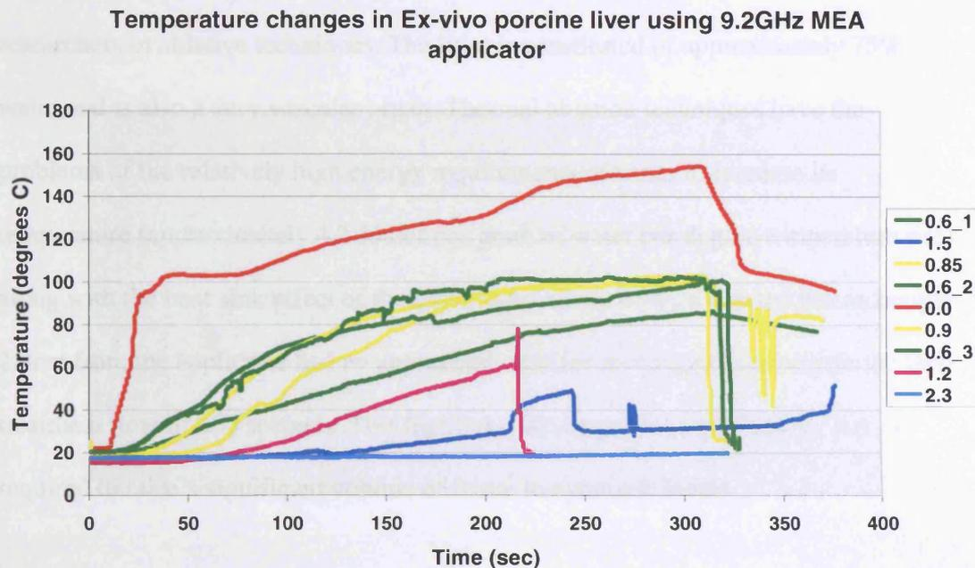
**Figure 3.** Temperature increases detected by thermocouples over a treatment time of 300 seconds using a 45 Watt, 9.2 GHz microwave system.
