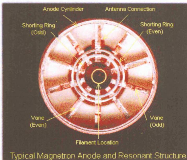
**Figure 2.6.** Schematic showing the internal structure of a microwave magnetron.
