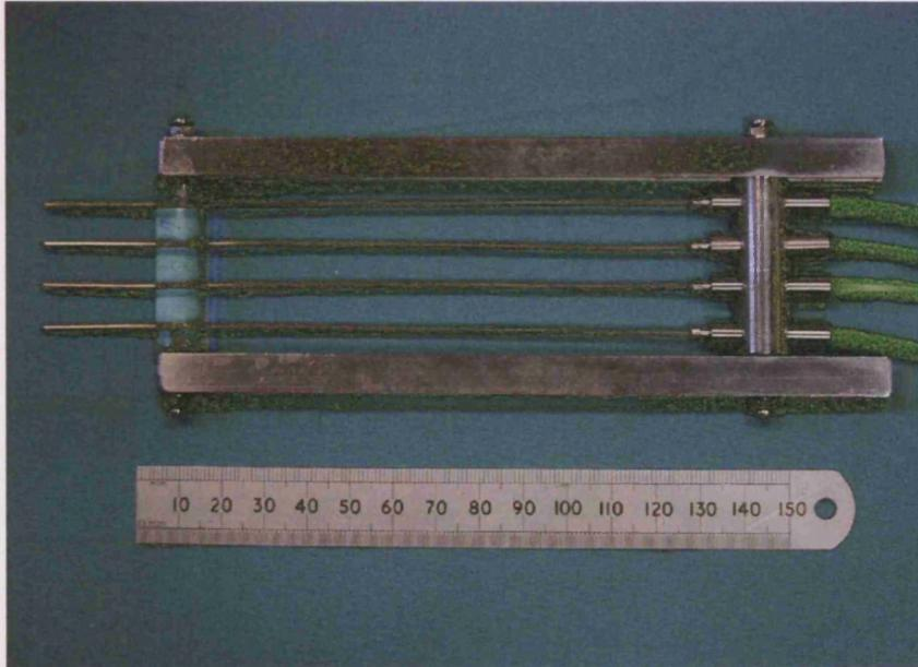
**Figure 1.** Aluminium jig constructed to house the thermocouples used for real-time temperature measurements. The thermocouples can be seen protruding from the left edge of the jig and could be buried into the hepatic parenchyma. The wires leading out from each thermocouple entered the data acquisition unit. The interval between each thermocouple is 1cm.
