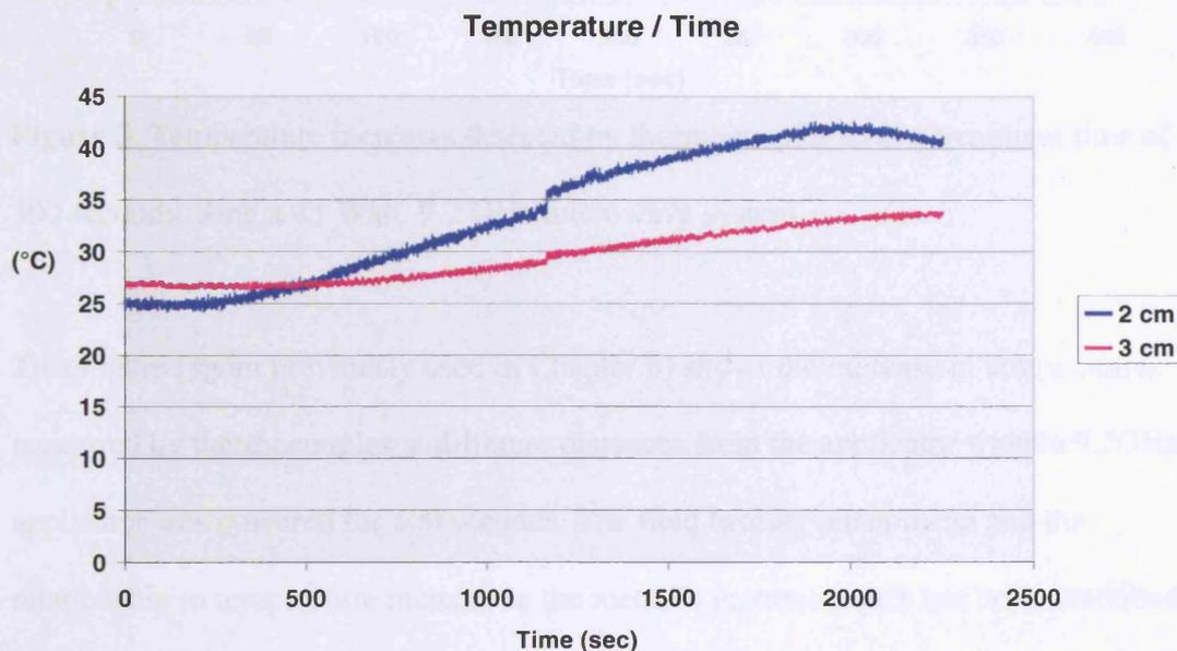
**Figure 2.** Increase in temperature in hepatic parenchyma following a microwave ablation of 40 Watts using the 9.2GHz microwave system. A steady rise in temperature can be seen in both thermocouples although the rate of temperature increase is greater in the thermocouple nearer the ablation centre.
