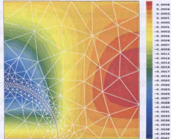
(b) Elastic displacements in the  $y$ -direction
