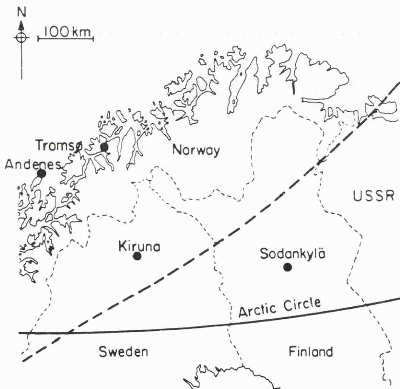
**Figure 4.1** Sketch map of EISCAT. The UHF transmitter is at Tromsø, the receivers are at Tromsø, Kiruna and Sodankylä. The dynasonde, an ionosonde, the partial reflection experiment (PRE), optical and magnetic instrumentation are also at Tromsø. The dashed line shows the southern boundary of the auroral oval under quiet geomagnetic conditions at 00h UT (after Rishbeth and Williams 1985).
