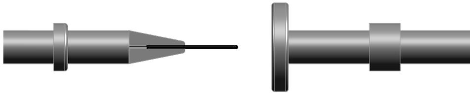
Figure 3.5: Physical implementation of the plane-tip electrode array. The tungsten tip (in black) has been spot welded on to the stainless steel pin. The flat electrode is grounded and the tip can be either at positive or negative polarity with respect to ground; in our experiments the polarity of the tip was chosen negative.
