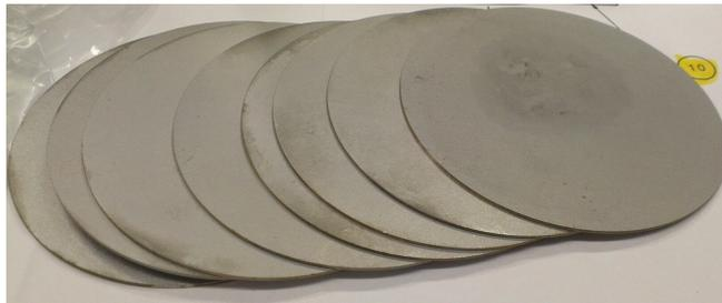
Figure 3.34: PADD1 1 mm thick 99 mm diameter 99.997 % pure tungsten filters (8 in total). The housing has room for an additional 2 filters however Goodfellow did not have the entire set in stock prior to the preliminary fielding, and the full compliment were not necessary for the August 2014 experiments.
