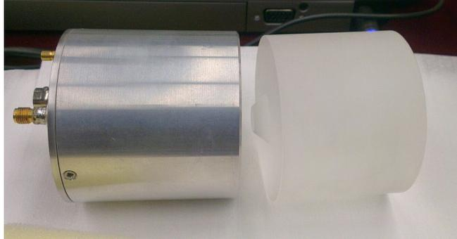
Figure 3.33: Photo of the PADD1 5 cm glass and PMT de-coupled to allow observation of the input window conical protrusion used to couple the Cherenkov light to the PMT input window.
