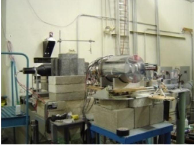
Figure 2.5: Photo of the HI $\gamma$ S NaI(tl) array used as the flux benchmark for cross-calibration with the plastic paddle detectors.
