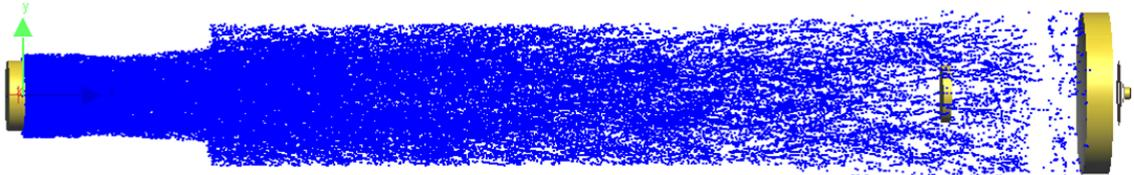
Figure 3.43: Image produced by LightTools showing the starting locations (blue from GEANT4) in GCD1 for a gas pressure of 100 psia in CO<sub>2</sub>.
