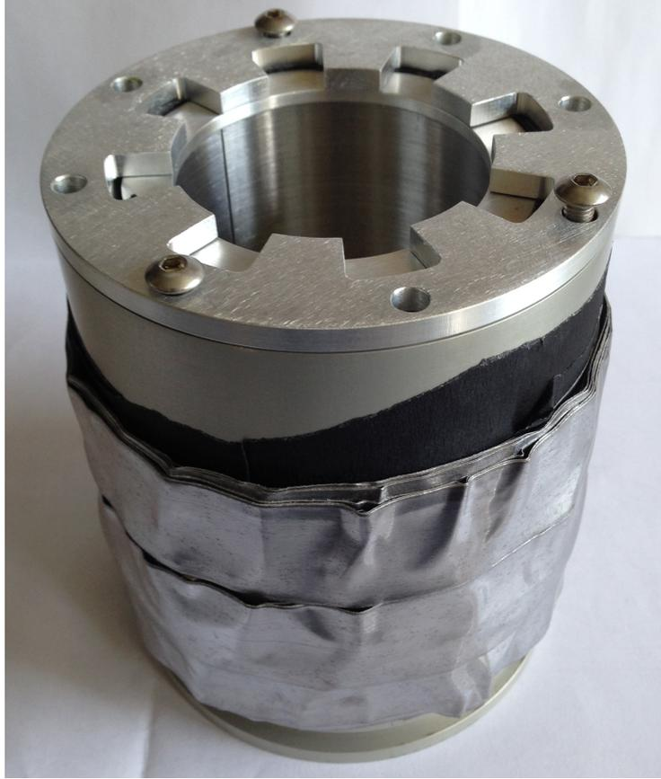
Figure 3.40: Photo of the PADD1 detector with the full compliment of lead tape after A. Zylstra’s astrophysics campaign. The black tape was used to ensure the housing was light tight subsequent to the PMT change on F. Merrill’s shot day.
