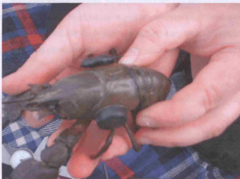
Plate 2.1.1: Photograph of a TW-4 (392Ag cell) radio transmitter and plastidipped Ibutton temperature data logger glued to a Signal Crayfish.
