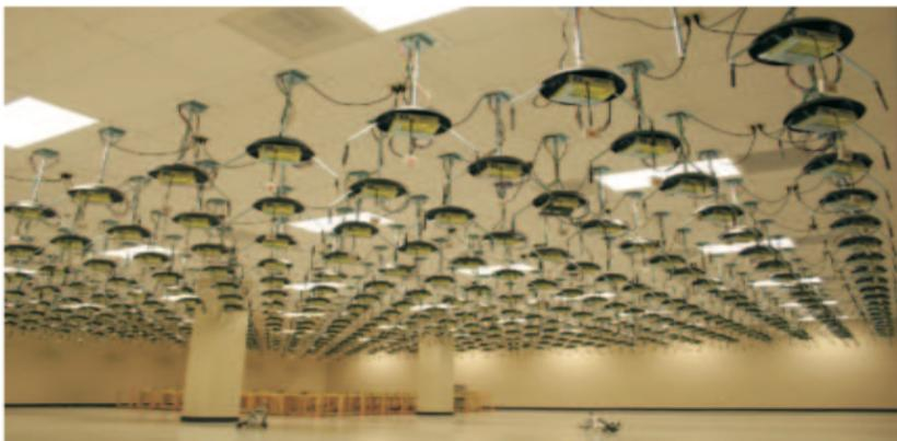
**Figure 6.4: ORBIT testbed grid of 400 nodes (from [Raychaudhuri05])**
