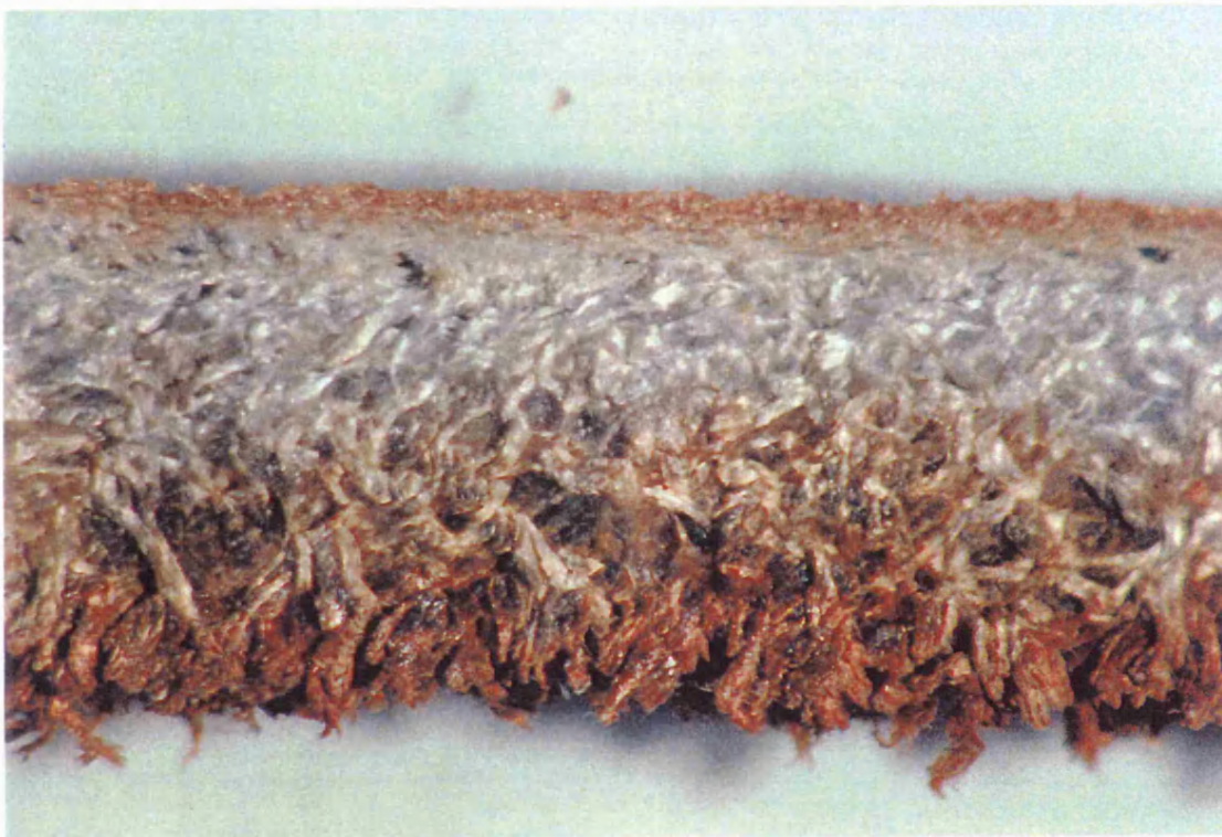
Fig. 3.39 Optical micrographs of resin retanned wet-blue dyed with (bottom) and without (top) ultrasound (50°C, 100 minutes, Airedale brown 3RG, magnification \times 25 )
