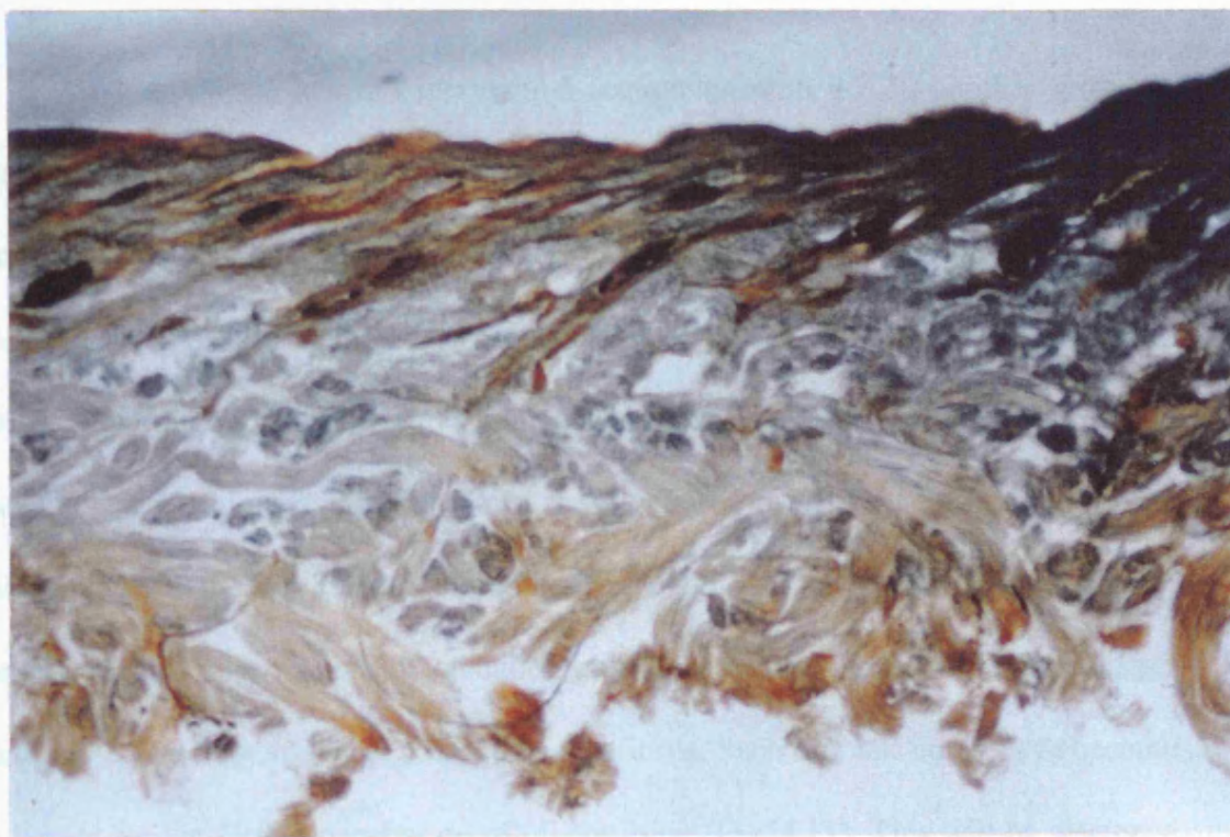
Fig. 4.10 Optical micrographs of oil distribution within the cross section of leather fatliquored for 60 minutes at 40°C (A-with ULT, B-without ULT; magnification x30)
