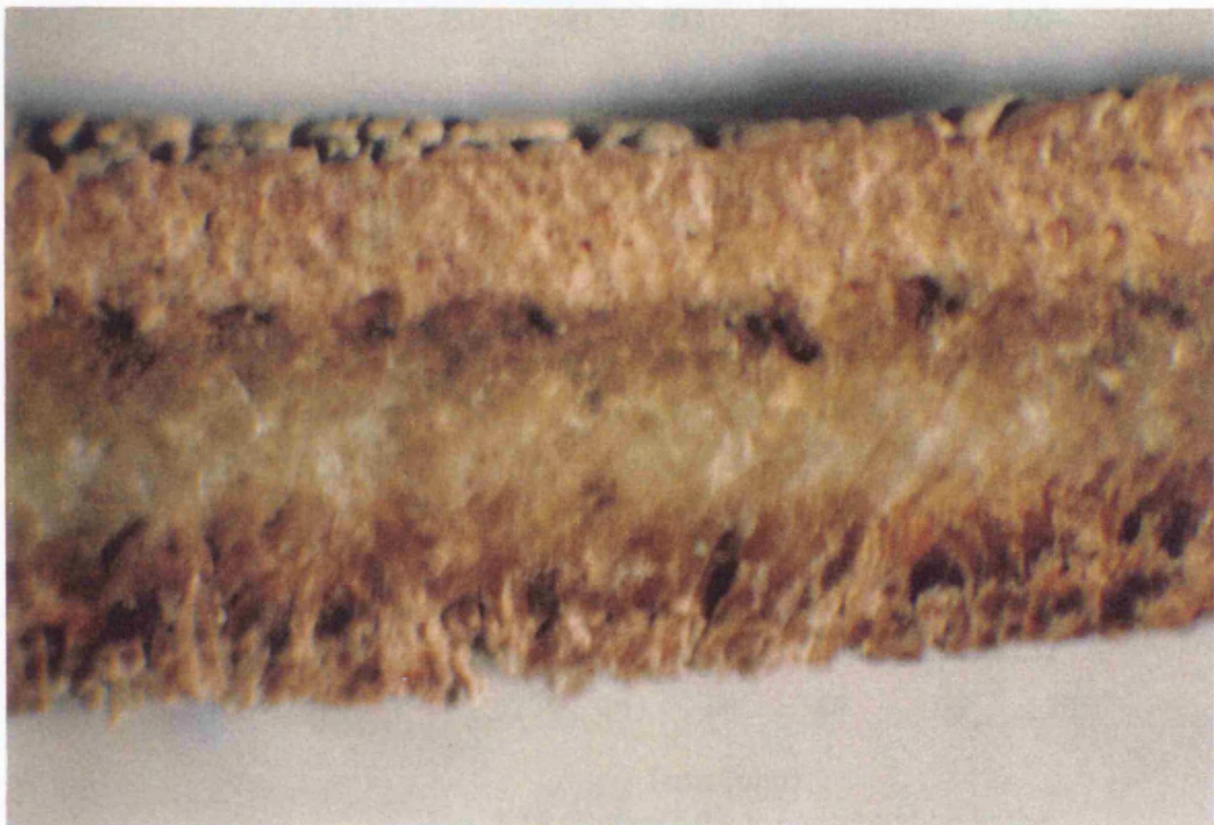
Fig. 5.15 Optical micrographs showing tannin penetration in sample 3 (magnification, \times 30 )
