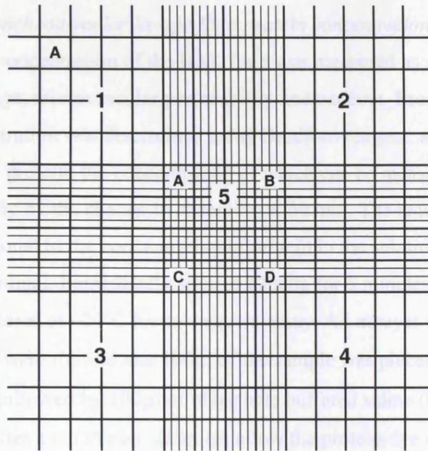
The solid black lines are in fact triple lines. The white cells are counted in squares 1, 2, 3 and 4. Red cells and platelets are counted in squares 5A, B, C, D, E.
