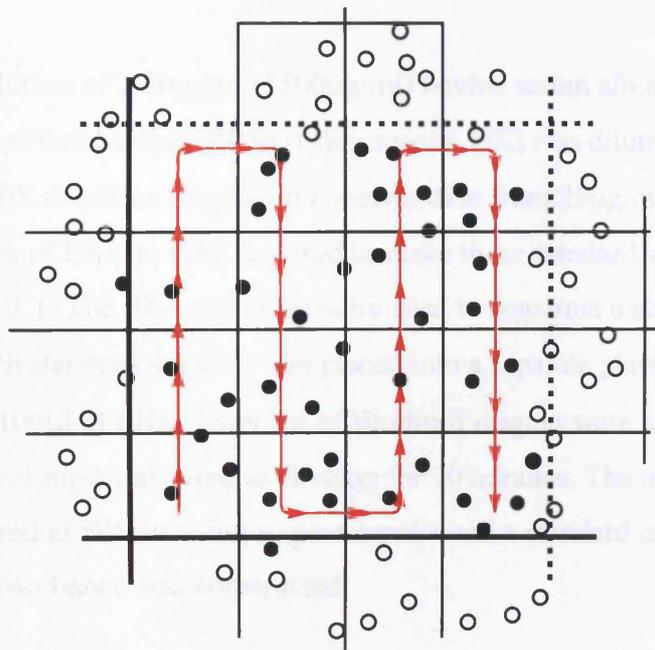
Counting sequence. A diagrammatic representation of the white cell count, showing the sequence of counting which should be followed, the square shown is 1. The same sequence of counting would be followed for any squares 2, 3 and 4.
