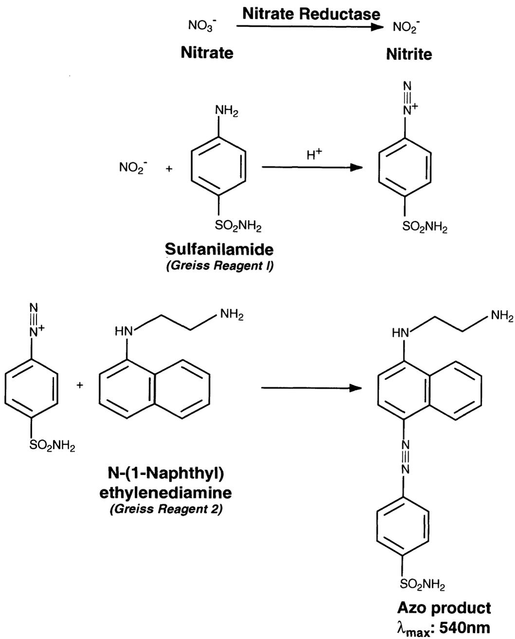
Figure 3.8 Biochemistry of the Greiss Reagent assay
