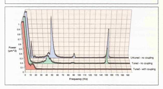
• An Anti-Vibration Coupling: A wide range of compliant materials were tested for their dampening capacity by sandwiching them between two brass plates in series with the motor shaft. The materials included rubber, foam rubber and anti-vibration mount cut to different
