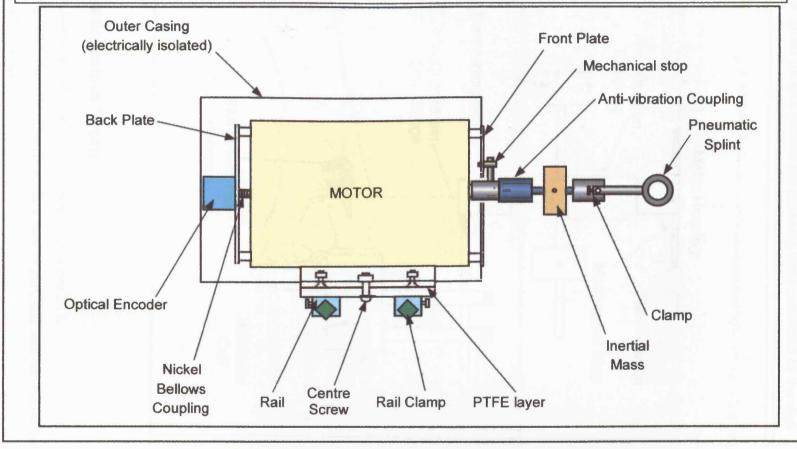
**Figure 2.12.** An outline diagram of the digit attachment to the motor shaft. The range of motion is restricted using electrical (microswitch) and mechanical stops. An antivibration coupling reduces unwanted vibration. Counterbalances act to balance the weight of the pneumatic splint into which the digit fits. Strain gauges records the opposing force generated by the digit.
