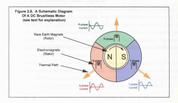
DC brushless motors have successfully been used to apply movements and impose various load conditions to human finger joints (eg. Al-Falahe & Vallbo, 1988, Vallbo & Wessberg, 1993). Previous system have been custom built by control systems specialists, but more recently, 'off the shelf' control modules have become commercially available, which allow the layman to set up and control DC brushless systems. The advantages and disadvantages of a DC brushless system are:
