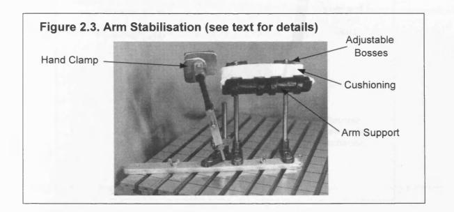
Hand Clamps and Supports: Hand stabilisation was critical for measuring tremor in the digits. A hand clamp was specifically constructed to provide:
