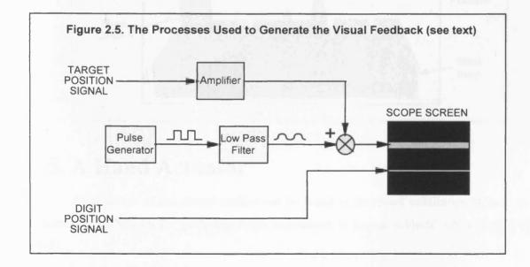
A target voltage signal was generated using a sequencer program created in Spike2 for Windows<sup>®</sup> (Cambridge Electronic Design). The gain or amplitude of the target movement could be controlled using an amplifier. To distinguish the target signal from the digit position feedback, a quasi-sinusoidal signal, generated using a pulse generator and a variable low pass filter, was added
