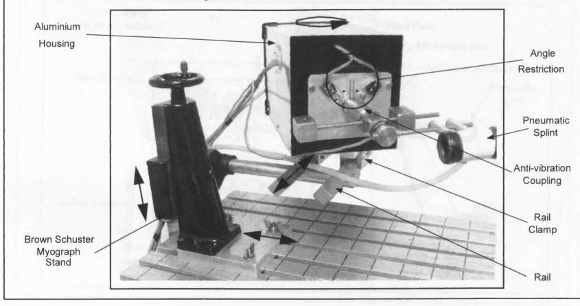
Figure 2.11. A Schematic Diagram Of The Actuator: An optical encoder is fixed to the rear plate of the motor and connected to the motor shaft with a nickel bellows coupling. At the front of the actuator, mechanical stops restrict the range of motion. The pneumatic splint is connected to the motor shaft via an antivibration coupling with inertial masses to dampen vibration. The foot of the motor can rotate aided by a low friction PTFE layer. Rail clamps hold the actuator on the bottom rails.
