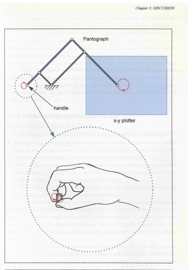
Figure 5.3. A method for applying 2-dimensional movements to the digit tips. A pantograph scales down movements generated using an x-y plotter. The subject senses movements through a handle attached to the end of the pantograph.
