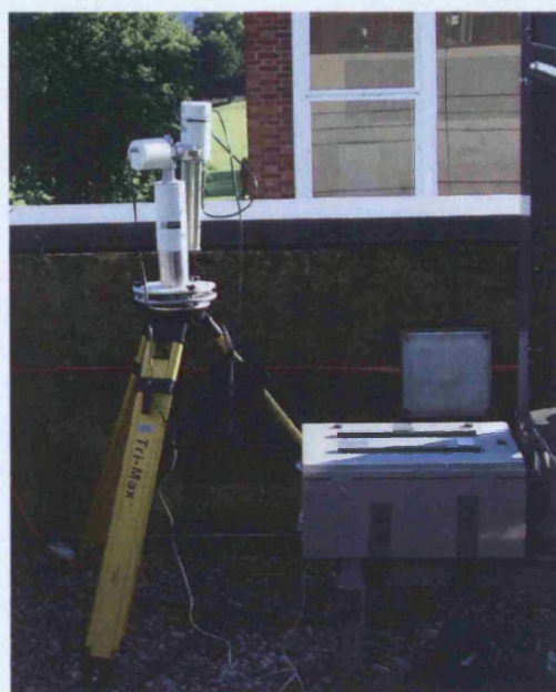
Figure 1-8: CIMEL sun photometer operating at the University of Leicester in 2007.
