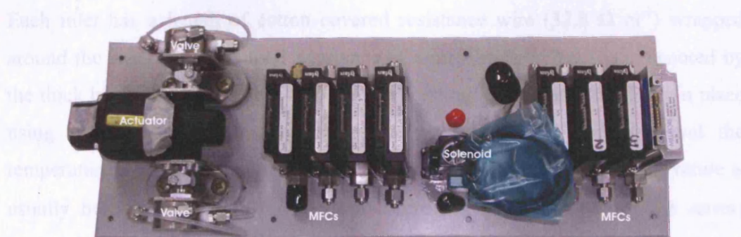
Figure 2.5 – MFC tray showing mounting of MFCs, solenoid valve and pneumatic actuator
