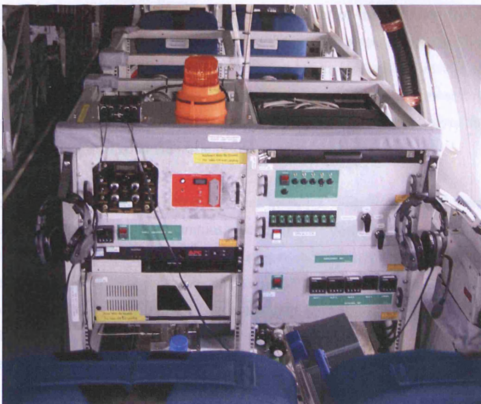
Figure 2.18 – Main and gas racks installed on the BAe-146
