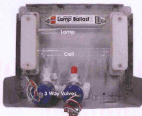
Figure 2.10 – Internal view of aircraft calibration source
