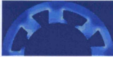
(a) Stator maximum  $B_{MOD}$  distribution
