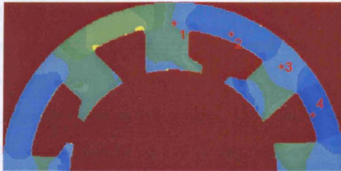
(a) Positions in stator for which flux orientation is compared
