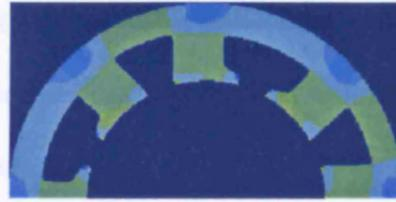
(b) Stator maximum  $B_{MOD}$  distribution
