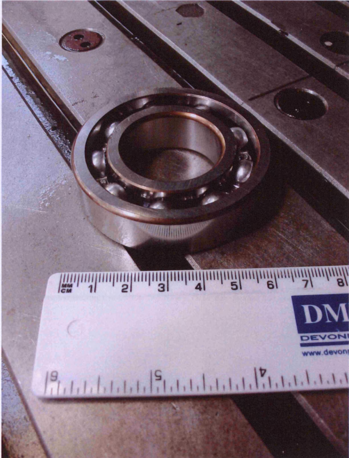
Figure A-6 Barden Bearing Ceramic Bearing at High Vacuum (HV) and Low Vacuum (LV) ends of iGX100 Dry Vacuum Pump.
