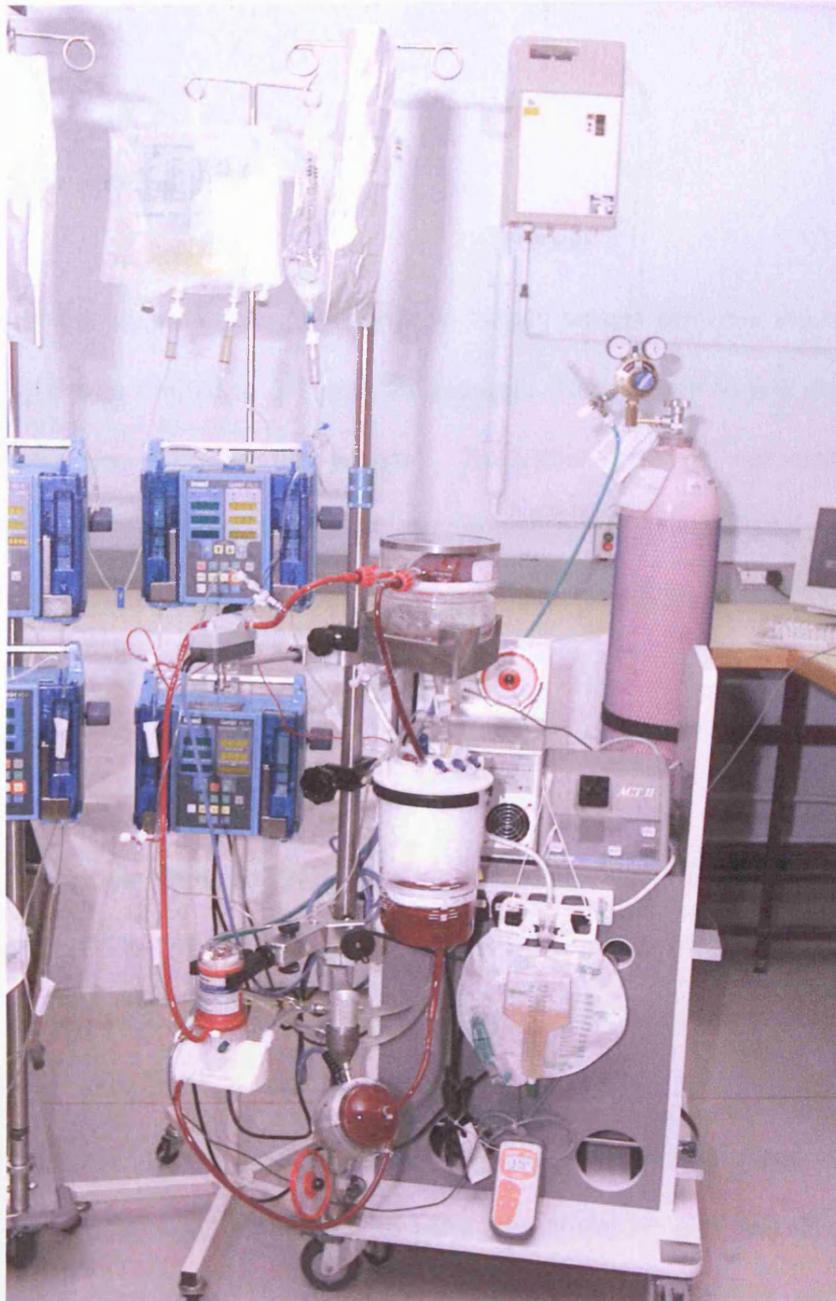
**Figure 1b:** Photograph of the Isolated Organ Perfusion System (IOPS)
