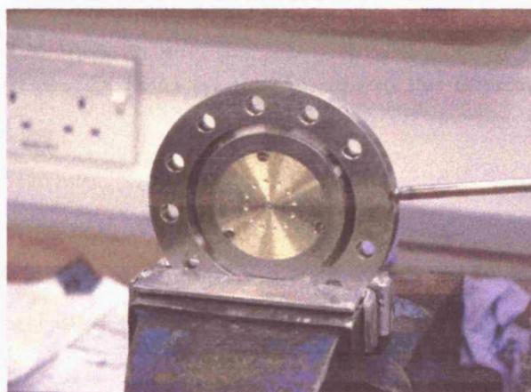
Figure 2.7 The Venturi flange.
