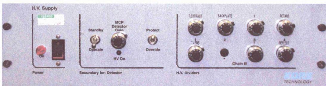
Figure 2.22 The Bias Control Panel of the TOF.
