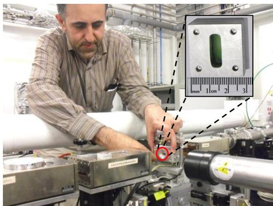
**Figure 2.5:** *Experimental set-up at BM25A, including sample stage, sample holder and both detectors. The fluorescence detector is centre and back, with black ring around end. The transmission detector is at the far left.*
