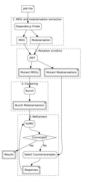
Figure 2. Data flow for the experiments; rounded edges indicate processes and the sheet icon indicates data - doubled icons signify plurality.
