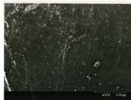
FIG 3b – SEM image of microwear on a cast made from a Speedex Light mould
