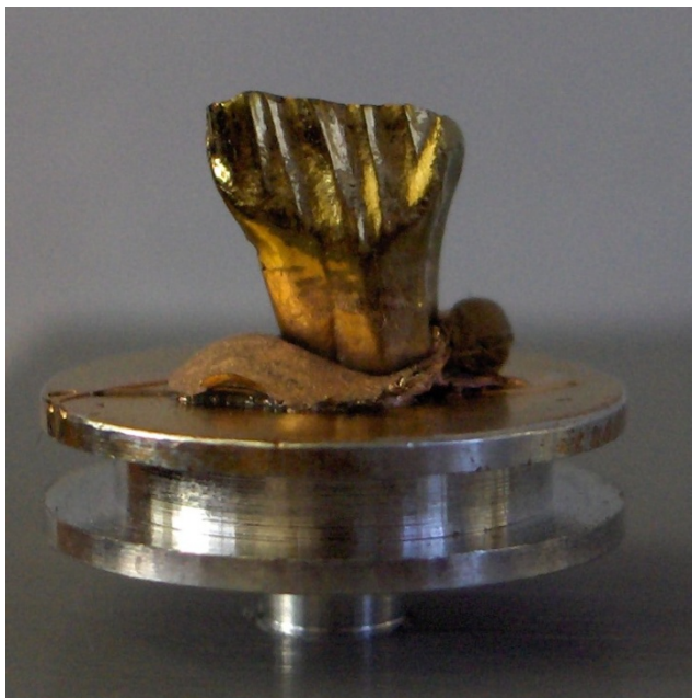
Fig 1c - Araldite 20/20 cast of a tooth from the ornithomimid dinosaur Hypsilophodon foxii , made from a Speedex Light mould, then mounted on a SEM stub and sputter coated with gold.
