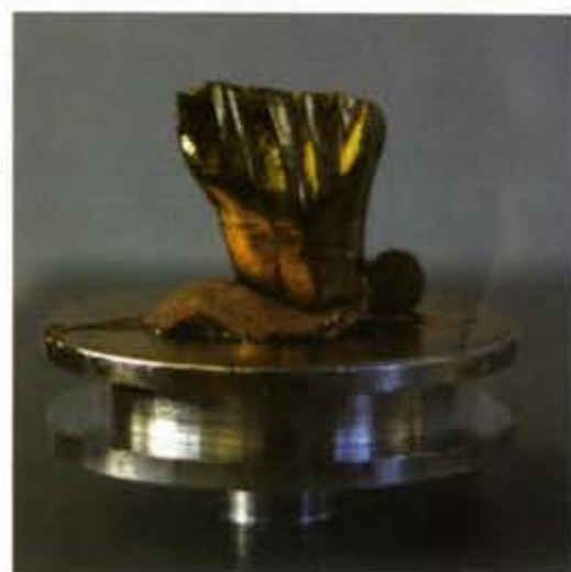
FIG 1c – Araldite 20/20 cast of Hypsilophodon foxii tooth, made from Speedex Light mould, mounted on SEM stub and sputter-coated with gold
