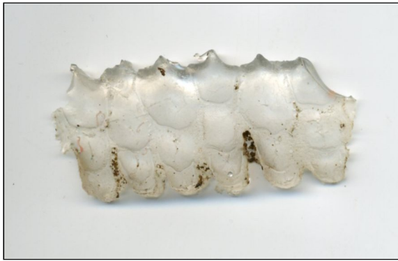
Figure 4. Transparent Araldite 2020 cast. This will be sputter coated in gold before imaging in the SEM.
