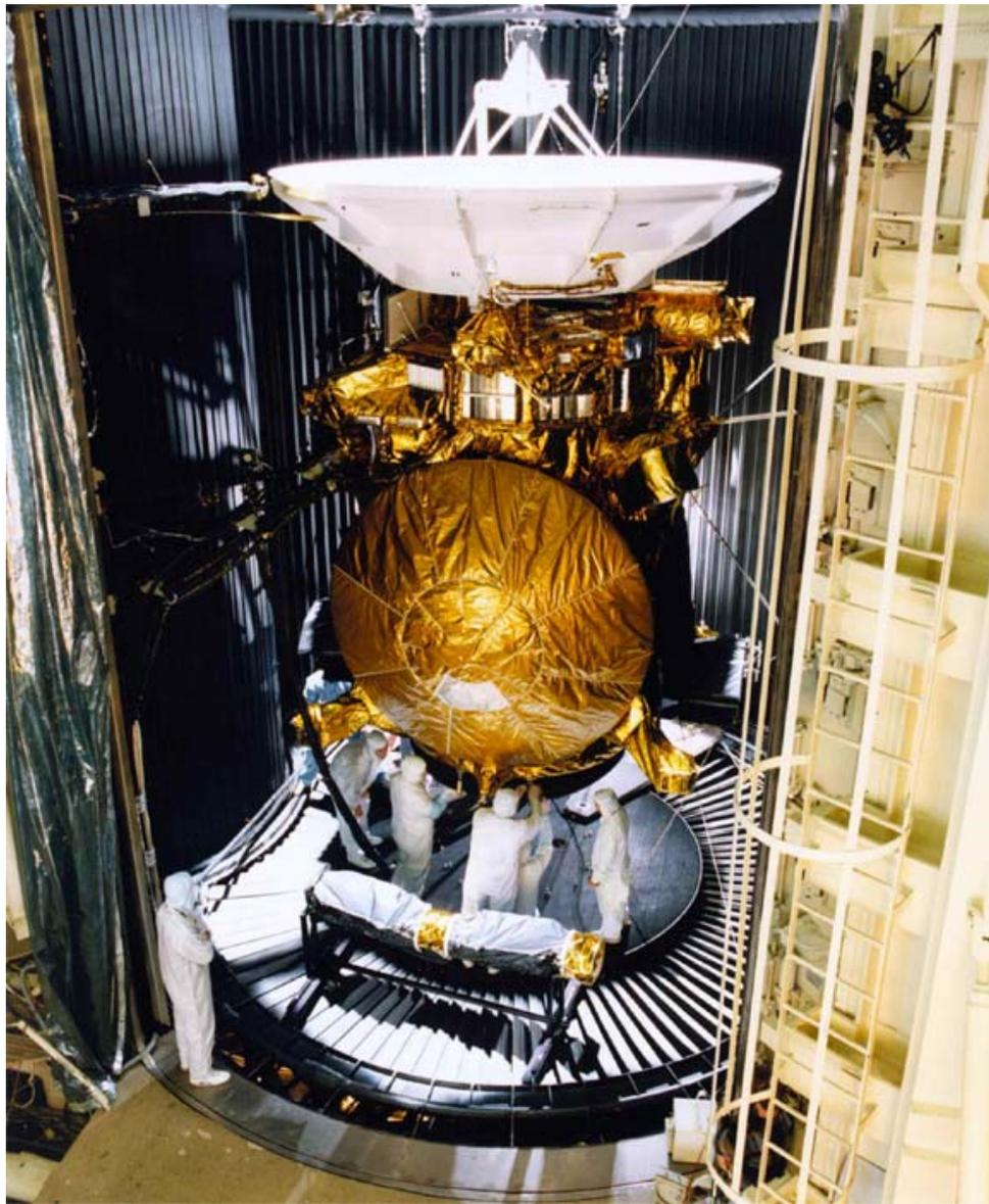
**Figure 3.1.** The Huygens probe (gold dome) being mounted onto the Cassini spacecraft.
