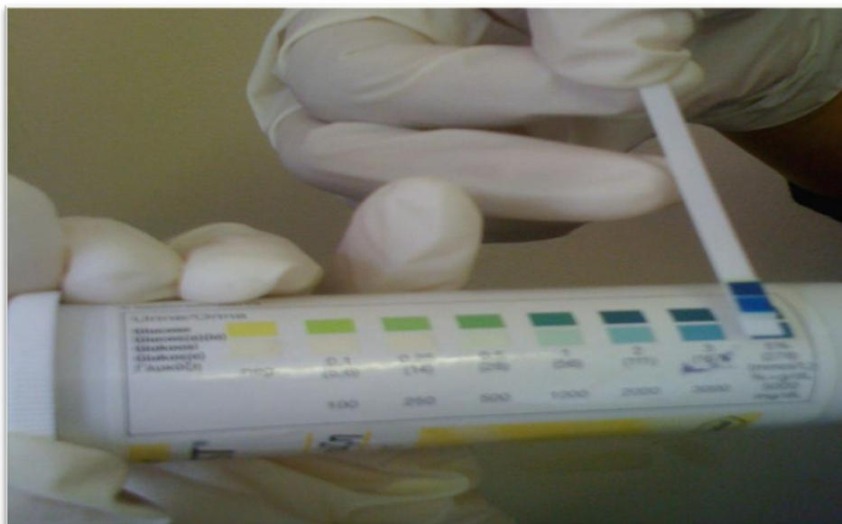
Figure 2.1 Test strip assay of HPD glucose levels using the DIBUR-TEST 5000 Glucose measurement kit
