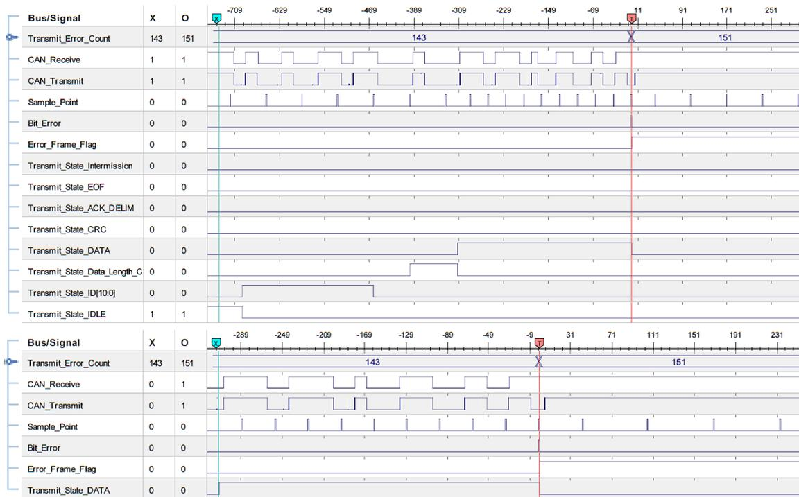
Figure 6.7: Error signalling and switch back in overclocked CAN
