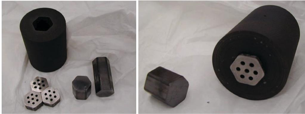
**Figure 5.13:** SPS bonding die designed and used by the author to join encapsulates and fuel cermets via diffusion bonding enhanced by SPS.
