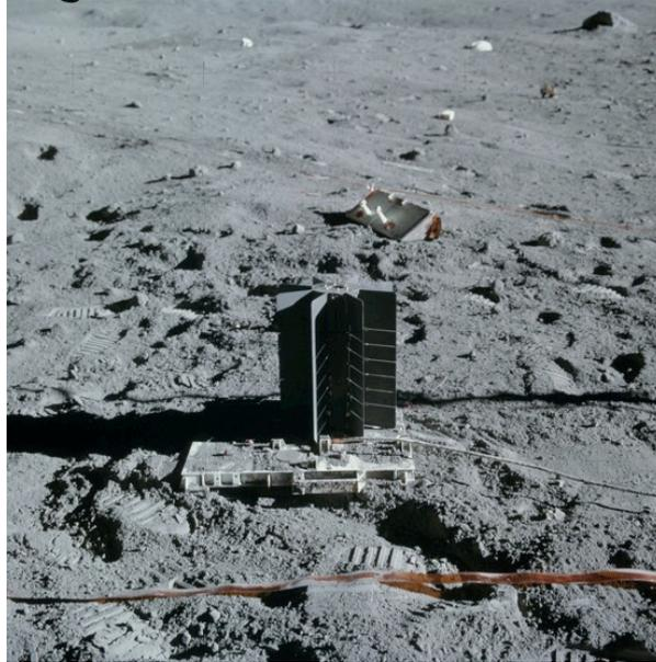
**Figure 2.6:** SNAP-27 RTG deployed on the lunar surface during the Apollo 16 mission [7].
