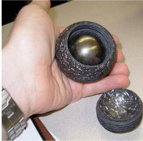
**Figure 2.8:** Image of the author holding a single Multi-Hundred Watt RTG heat source engineering model.
