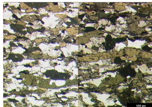
Figure 2.10. Subidiomorphic elongate amphibole grains forming a fabric with quartz and altered feldspar grains. Small rounded apatite grains can be seen in some amphibole grains. (*Sauda Grey Gneiss - Fine-grained aphyric diorite gneiss, SA7-77*)
