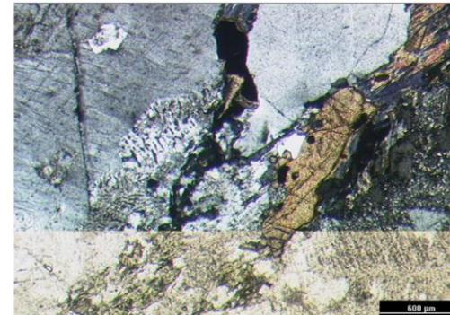
Figure 2.22. Myrmekite development (left of centre) on edge of K-feldspar, anhedral titanite grain (right of centre), and chlorite after biotite (top right).
