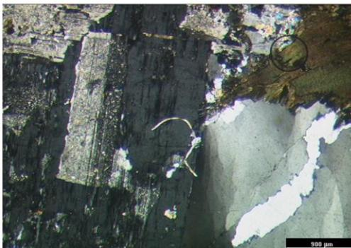
Figure 2.21. Deformed biotite grain surrounded by finer biotite grains (top right), altered and twinned plagioclase (left of centre), surrounded by perthitic feldspar, and quartz grain with undulose extinction (bottom right).
