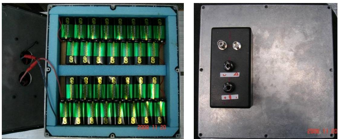
Figure 3.30 Photos of high voltage battery supply
