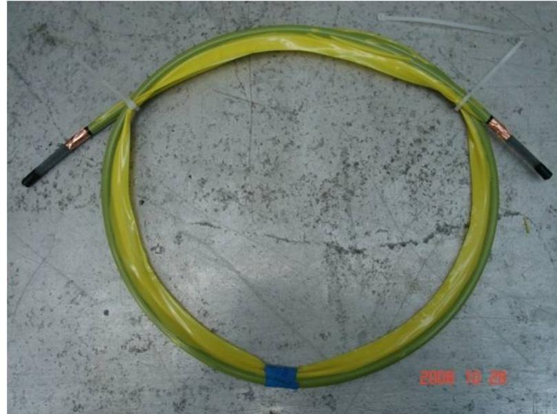
Figure 4.10 Test sample for conductivity measurement of semicon layers
