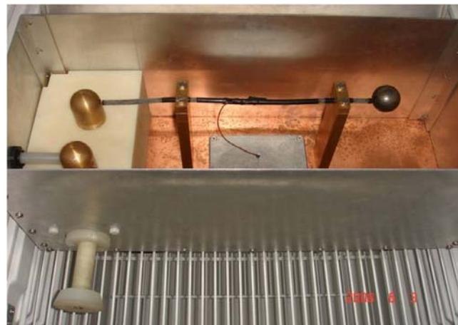
(b) photo of the test unit containing high voltage switch and a cable sample
