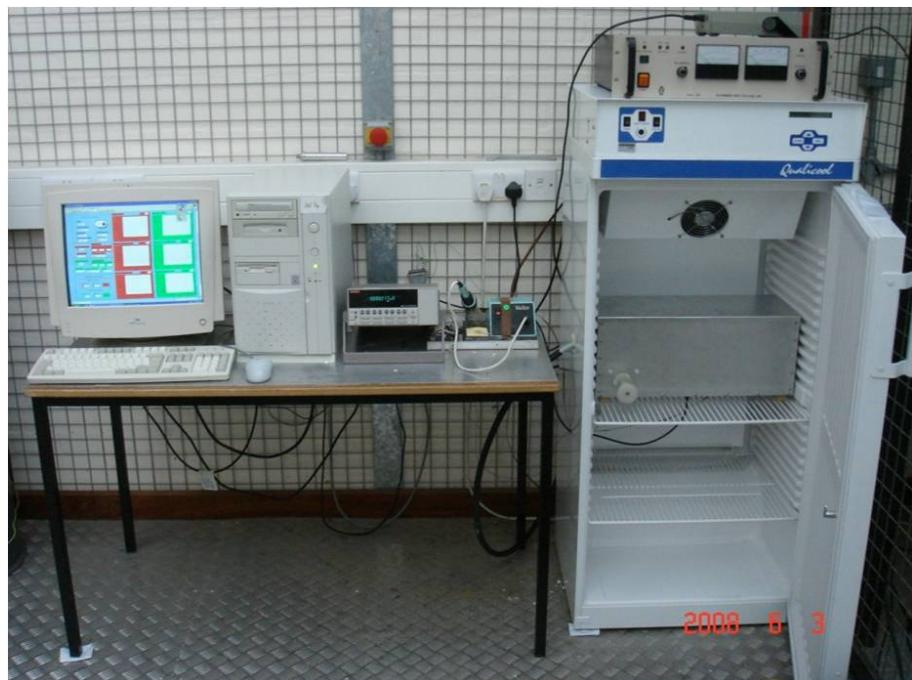
Figure 3.24 Charging/discharging experiment system with picoammeter
