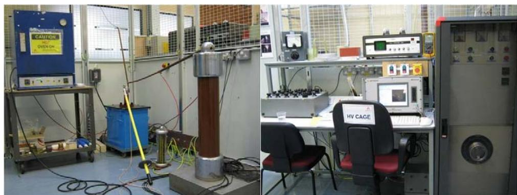
Figure 5.17 Schering bridge system setup. High voltage part in the left photo and low voltage control part in the right photo.
