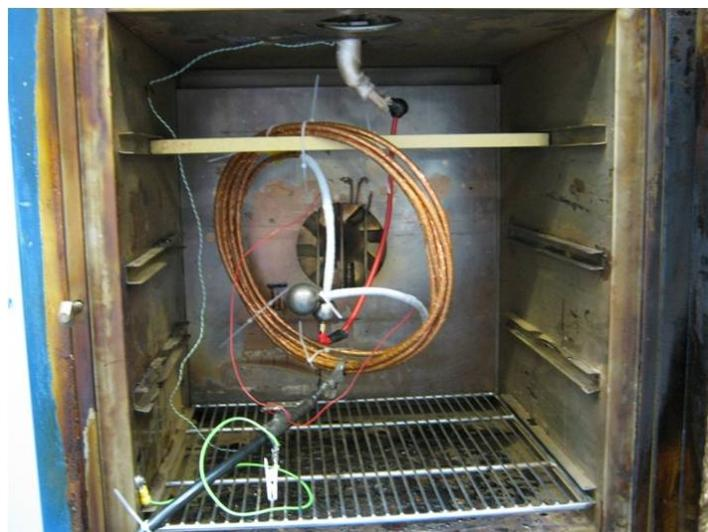
Figure 5.19 Cable sample in the oven for Schering bridge measurement
