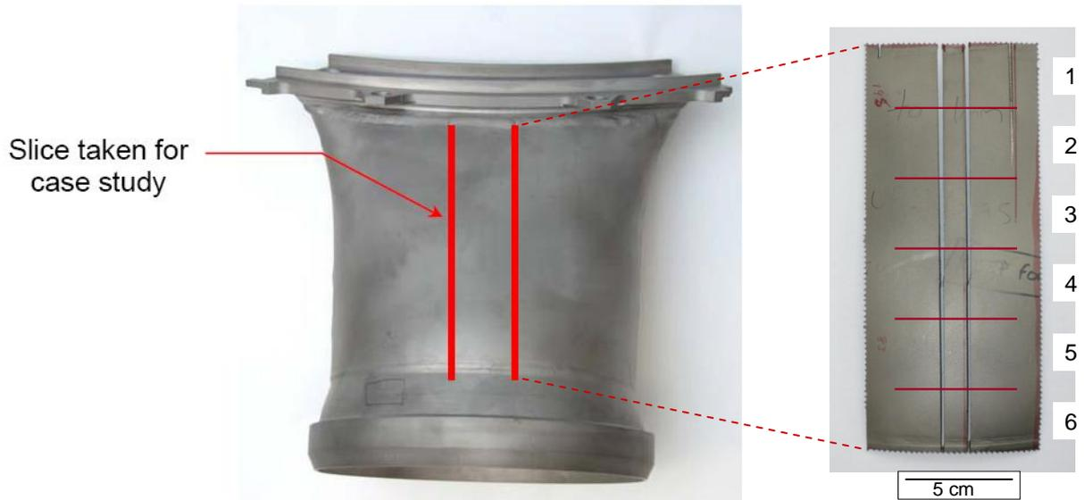
Figure 5.3 Location of the slice taken for metallurgical examination and illustration of its sectioning.
