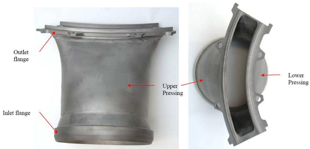
Figure 5.1 Typical views of The Transition Duct.
