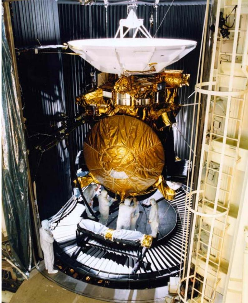
**Figure 3.1** The Huygens probe (gold dome) being mounted onto the Cassini orbiter.
