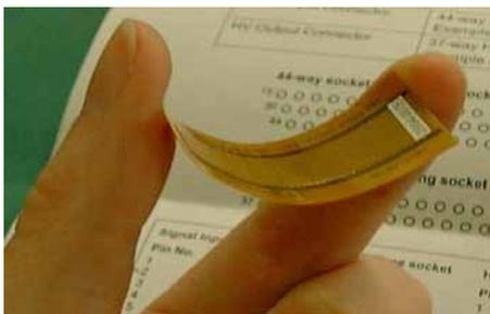
Figure 1.5: The flexibility of a piece of MFC. Image supplied by UCL.
