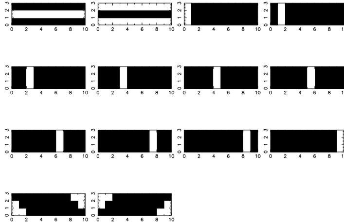
Figure 2.60: A series of fourteen local group patterns to control the piezoelectric devices during the X-ray tests. The white areas indicate the actuators which are active (with a value of +1) whilst the rest remain passive (with a value of 0). The voltage applied to each individual piezoelectric is calculated by taking these values and multiplying it by the voltage iteration value. Patterns three to ten are each of the columns of devices actuated in turn.
