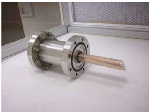
Figure 2.57: The copper anode of the X-ray source coated in a thin layer of NaCl to excite the emission lines required for the X-ray tests.
