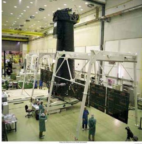
Figure 2.3: The XMM-Newton satellite during the solar array deployment test at ESTEC, Netherlands[5].
