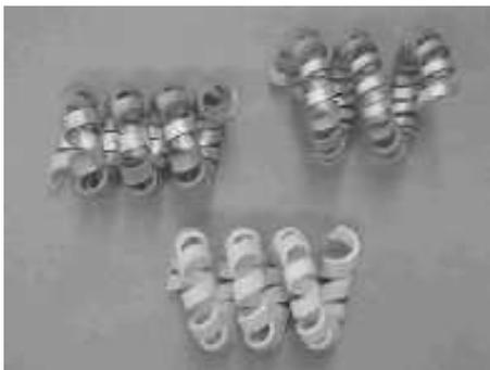
Figure 1.6: Examples of piezoelectric devices created at the School of Metallurgy and Materials, University of Birmingham.
