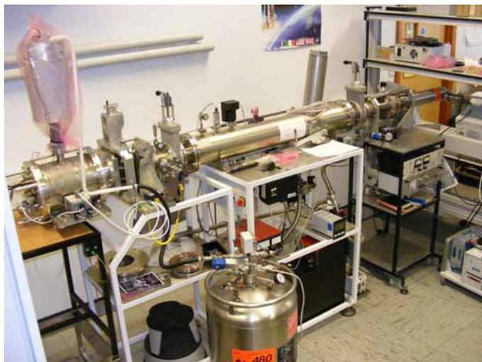
Figure 3.37: Image of the XMM-Newton CCD life test facility at UoL. The test facility is 3.1m long with an X-ray source, X-ray CCD and mounting at the centre, for an optic. The X-ray source is on the right hand side of the image (by the bookcase) whilst the CCD is on the far left of the image. The MOA was mounted behind the flange which is in the centre of the pipe. The rotation arm can also be seen attached to this flange.
