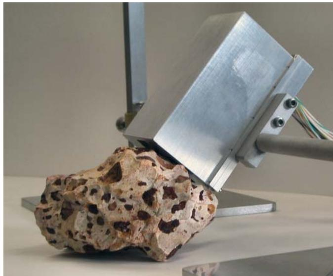
**Figure C.6** Beagle 2 Qualification Model (QM) Mössbauer sensor head (B2MBSS) in contact with test sample (not a GSPARC specimen). This configuration (backscatter mode) was used for all laboratory measurements. Sample is ~7 cm across. Courtesy Dr. Christian Schröder, NASA JSC.
