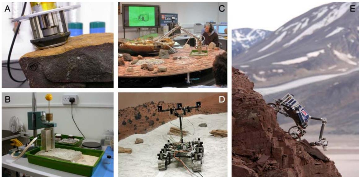
**Figure 3.2** Analogue field measurements performed in the lab with standalone instruments (A), tools (B), and robotic payloads (C). Mission-like complexity is further introduced during controlled trials in planetary yards (D), and ultimately, in the field (E). Courtesy NASA JPL (E).
