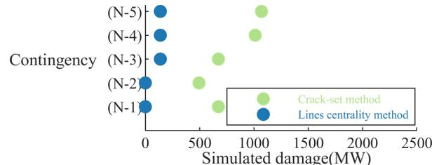
Fig. 13. Contingency comparison between the line centrality method and crack-set method for nest\_a\_case118\_ieee
