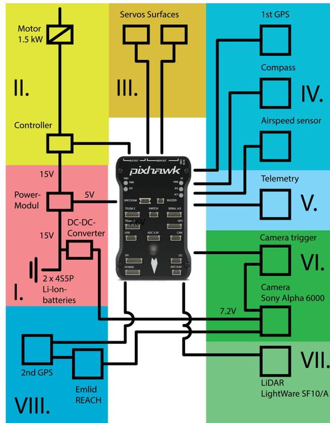
**Figure S1.** Layout of the UAV components around the Pixhawk autopilot.
