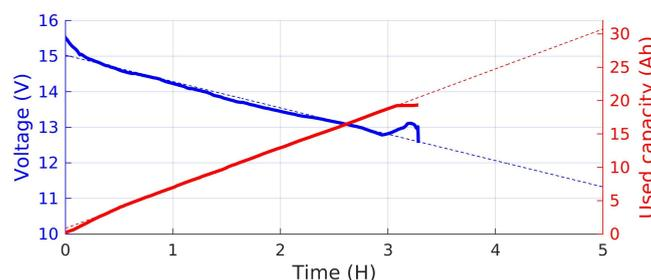
**Figure S2.** Battery voltage and used capacity during a 180-km long flight operated in the Inglefield Bredning.
