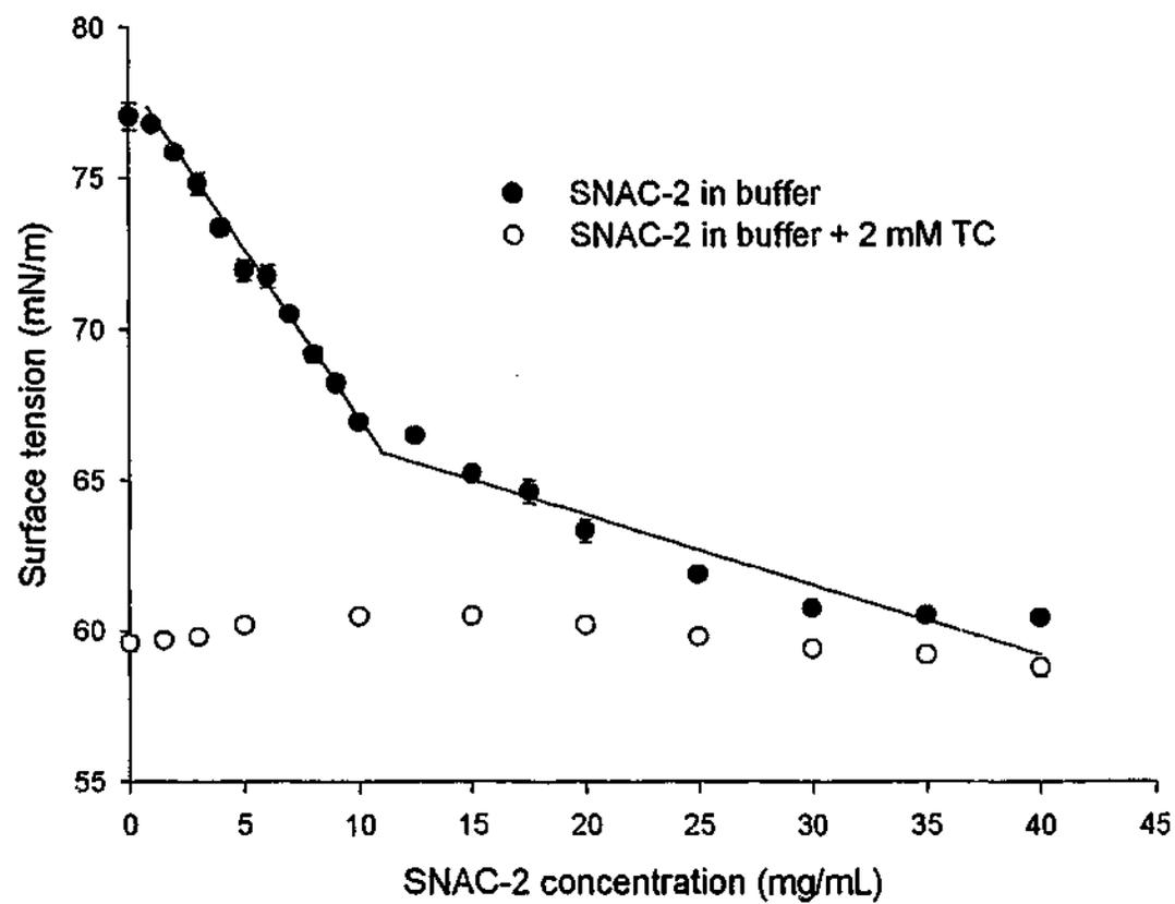
**Figure 6.1** Surface tension (mN/m) versus SNAC-2 concentration in modified diffusion buffer. Symbols represent the mean  $\pm$  SEM of three measurements.
