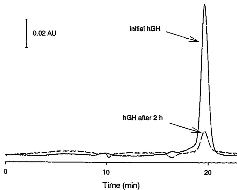
**Figure 5.5** Representative chromatograms of hGH in the initial and final donor solutions in the absence of additives during a typical experiment in the modified Ussing chamber. Chromatograms were obtained using the SEC assay as described in Section 4.2.3.4.
