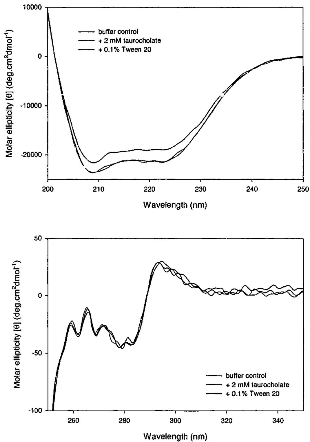
**Figure 5.9** Far (top) and near (bottom) UV CD spectra for hGH (0.5 mg/mL) in diffusion buffer in the presence and absence of excipients at 37°C. Spectra acquisition was accomplished using the method outlined in Section 3.1.2.2.3.
