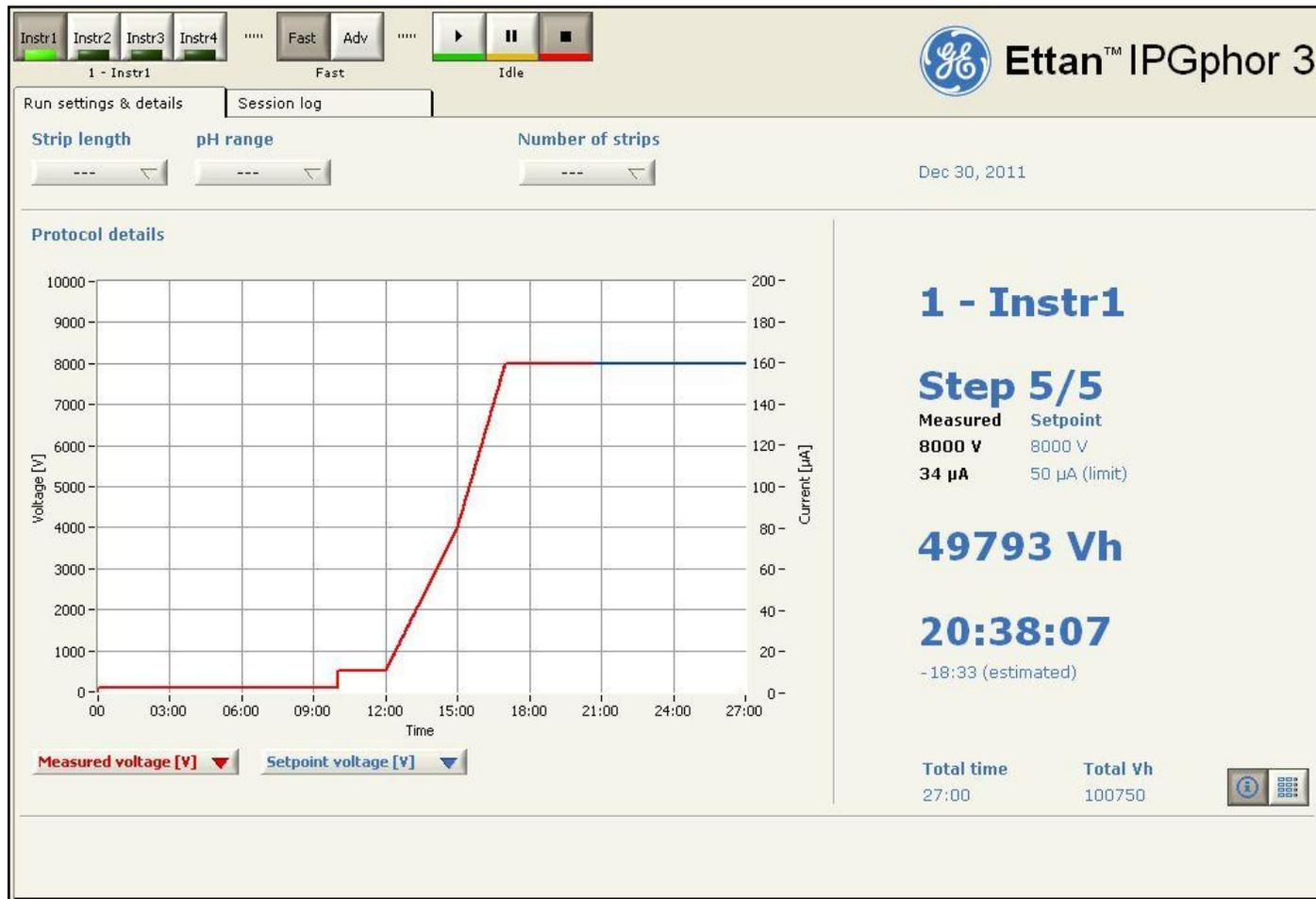
**Figure 3.2.2.** Graph showing the IEF running protocol on the Ettan IPGphor 3 apparatus. The blue line was the running protocol set on the instrument, whereas the red line recorded the real-time voltage and current during the exact run for monitoring purpose.
