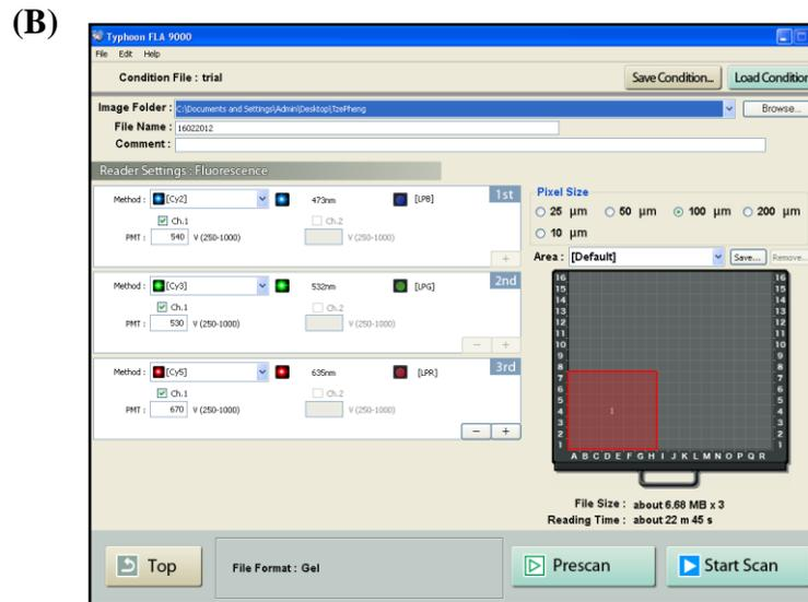
**Figure 2.2.1.** Typhoon Scanner Control windows. (A) allows mode and system settings, while (B) is for PMT voltage, pixel size, and area settings before gel scanning.
