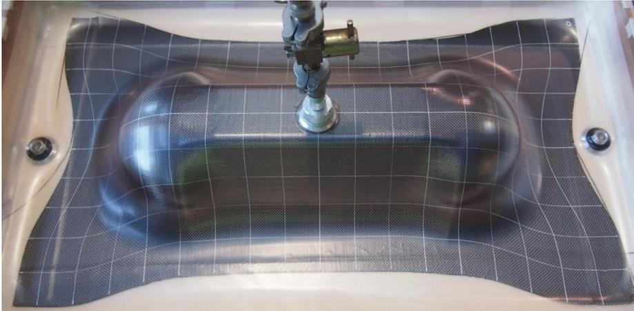
Figure 86: Carbon fibre fabric, formed to the double dome tool with 0°/90° orientation.
