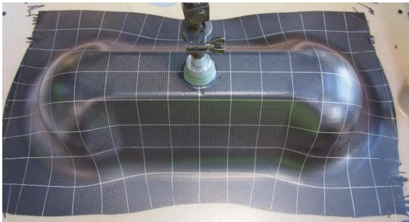
Figure 87: Carbon fibre fabric, formed to the double dome tool with -45°/45° orientation.
