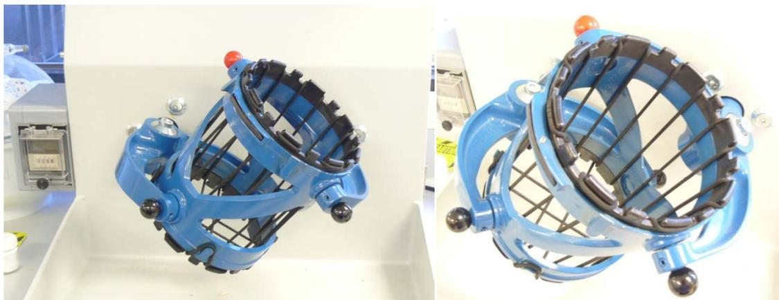
Figure 4.2: Turbula T2F tumbler (Willy A. Bachofen, Switzerland). Rotating arms hold each end of the drum with one arm (shown with red pin) mechanically driven. When operating drum is inverted and rotated in a “figure-eight” motion.
