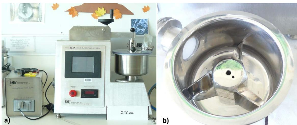
Figure 4.3: KG5 Laboratory scale mixer (Key International, U.S.A.). Mixer contains a variable speed motor with touch screen interface (a) and a standard 3-bladed inclined impeller within mixing bowl (b).
