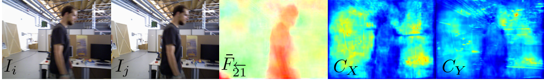
Figure 8.12: For a frame pair ( I_i and I_j ) from the sequence fr3-walk-xyz , \bar{F}_{ji}^L is the estimated optical flow from I_i to I_j , and C_x and C_y are the estimated flow confidences in the x and y direction respectively
