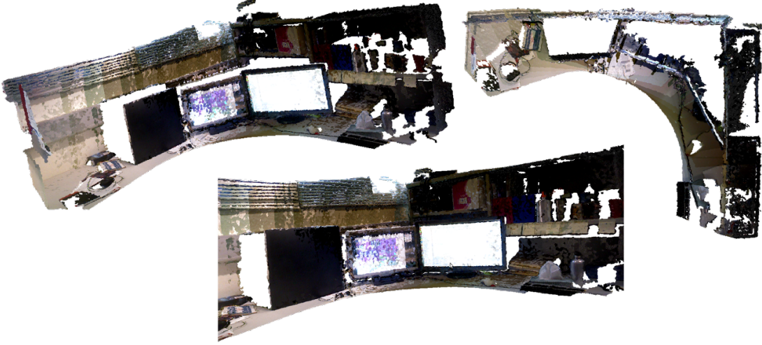
Figure 1.1: Demonstrates the alignment of multiple overlapping point clouds from a Kinect style depth sensor. Note the slight curve in the walls in the top-down view ( top-right ) caused by using an uncalibrated sensor to generate the point clouds. This alignment is performed using a dense implementation of point-to-plane ICP which is discussed in Section 3.7
