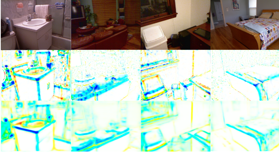
Figure 7.1: Top: The corresponding RGB image from the NYUv2 test dataset which was used as the only source of information to estimate curvature. Middle: The ground-truth curvature computed using the depth data using the approach from [24]. Bottom: The predicted curvature of this network. The false colouring is as shown in Chapter 5 and 6. Positive curvatures are shown in blue, negative in red, saddles in green and planes in white.
