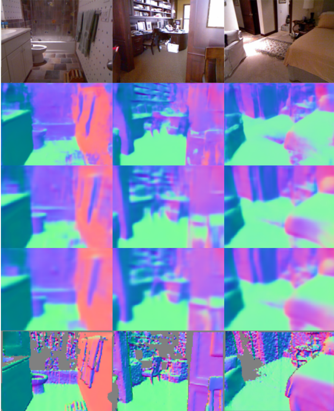
Figure 7.5: Demonstrates the qualitative improvement of this approach for normal estimation. Top: RGB image 2 nd row: Bansal[160], 3 rd row: Eigen[34], 4 th row: Prediction from this approach Bottom: Ground Truth [24]. The missing areas in the ground truth normals coincide with those in the raw depth images.
