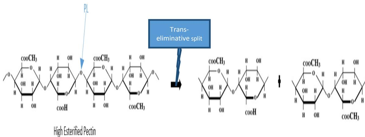
**Figure 5.** Catalytic activity of the lyases on esterified pectin- Modification of Jayani et al. (2005)
