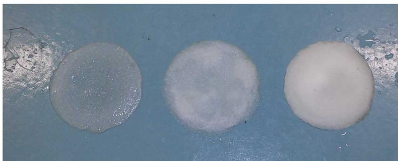
Figure 12 Digital images of wetted aerogels (From left to right: 0.0197 g/ml, 0.0239 g/ml and 0.0337 g/ml)
