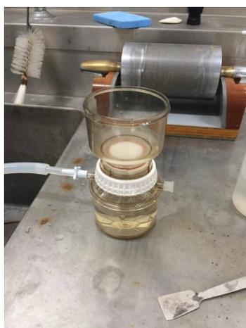
Figure 27 Experiment Set-up for filtration procedure to form the second layer
