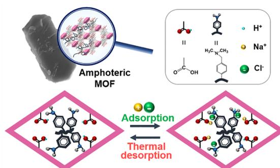
**Figure 6.1** Illustration of reversible ion sorption with functionalized MOF.
