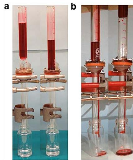
**Figure 3.17** Controllable oil-water separation using TPU-PNIPAM-3.6 membrane at (a) room temperature and (b) 45 °C respectively (hexadecane: red, water: transparent). Oil-water separation at 45 °C was conducted in a 45 °C oven.
