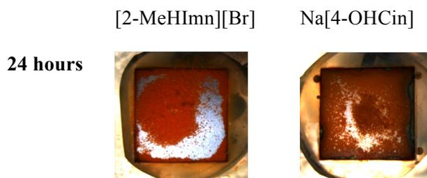
Figure S5. Optical images of steel coupons immersed in 4 mM solutions of component ion salts.
