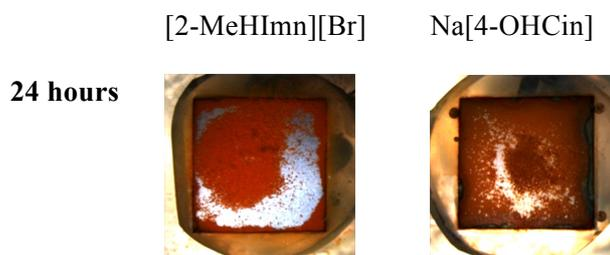
Figure S5. Optical images of steel coupons immersed in 4 mM solutions of component ion salts.
