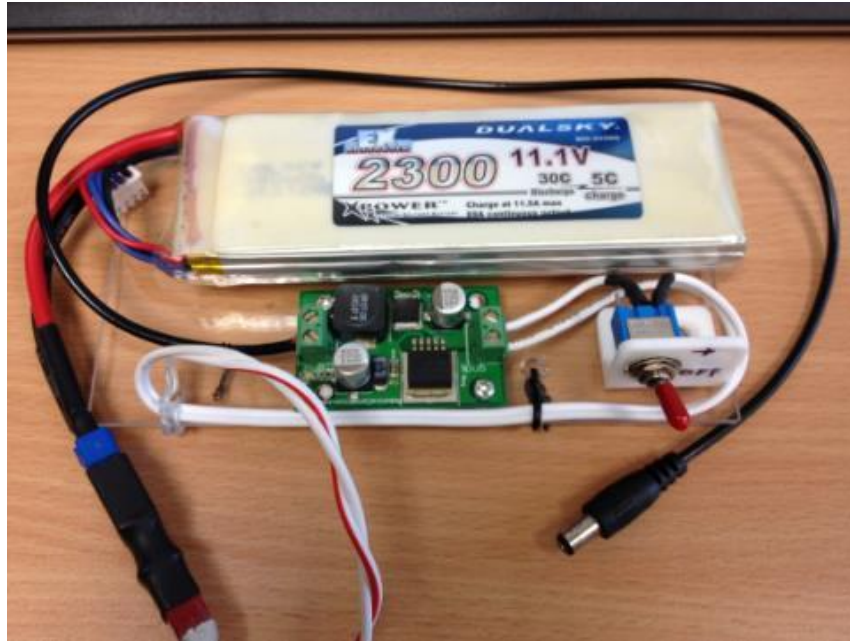
Figure A2.4: The lithium power source. Since ODROID XU3 is running on 5 volts, a voltage regulator (the green board) is added to convert the 11.1 volts from the lithium battery. Battery specifications: 11.1V, 2300 mAh, 30 C, Li-Polymer battery.
