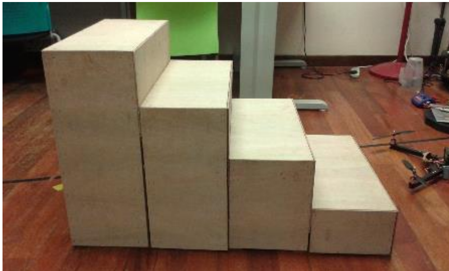
Figure 6.3: Adjustable blocks set for the lab test can be used to resemble stairs, rises, drop-offs, curbs and other forms of surface discontinuity.
