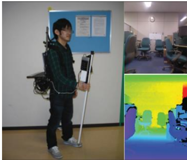
Figure 2.10: A depth sensing technology proposed by Takizawa et al. (2012) and Takizawa et al. (2013).
