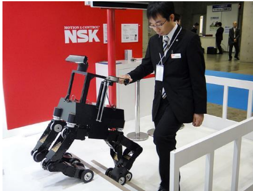
Figure 2.15: A four-legged guide-dog robot developed by NSK (2011) based on depth sensing technology, capable of obstacles and steps recognition.
