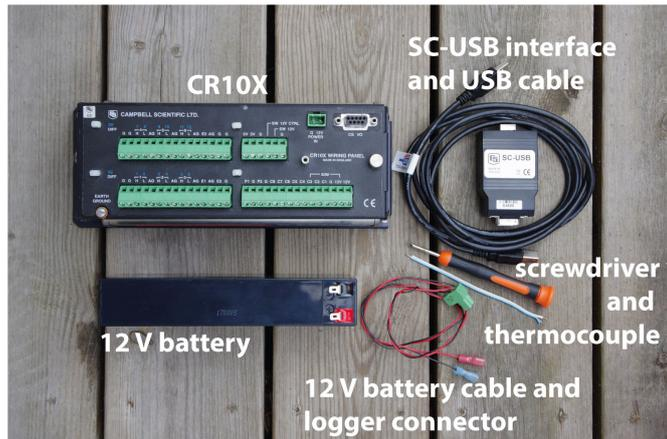
The logger consists of a wiring panel where sensors are attached and the encapsulated logger electronics, a steel can beneath the wiring panel. The panel and the logger can be separated although not unless necessary.
