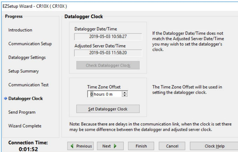
You will see the clock on the data logger and the clock on the computer or 'server'. If the logger time is off you can adjust it to the computer time by pressing 'Set Datalogger Time'. The two fields should now show the same time.
