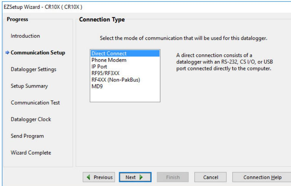
Only one option will be relevant here and it is the 'Direct Connect' which allows you to directly connect to the logger using an USB cable. Continue by pressing 'Next'.
