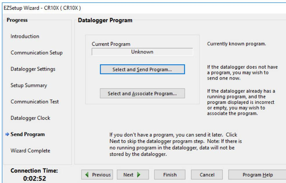
You have two options, either send a new program to the logger or just associate a program already on the logger to a file on the computer. This is necessary to allow variable name and other features in your logger program to be displayed correctly in the PC400 software.
