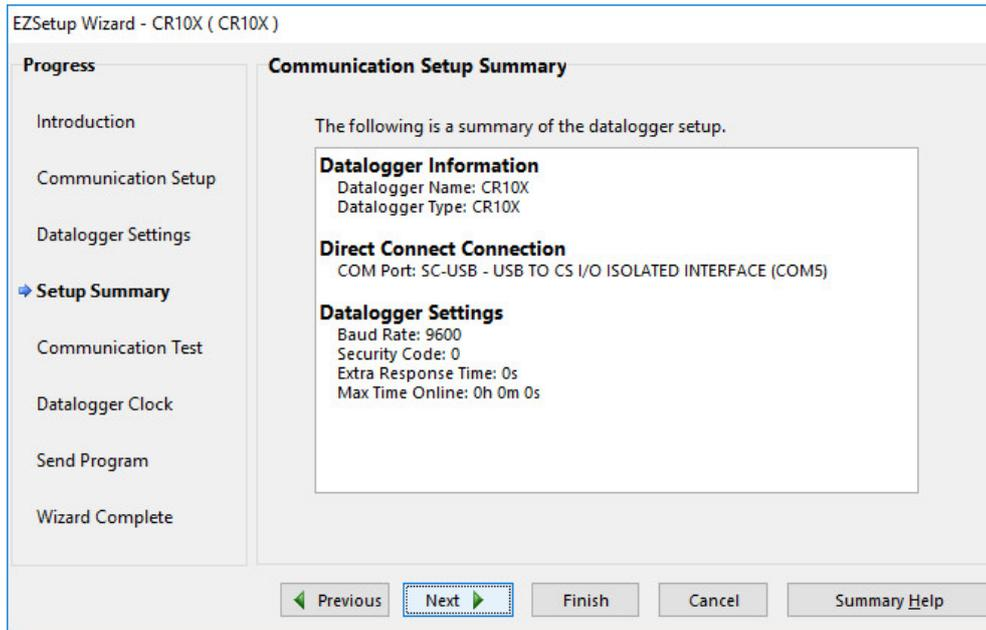
In this example you may note that the COM-port used by SC-USB has been named COM5. It is important to remember that this number is set by the software so it is not certain that the same port number will be used if you get back to the station later, particularly if you use a different USB port on the computer. You can always change the port settings if you find you cannot get a connection.
