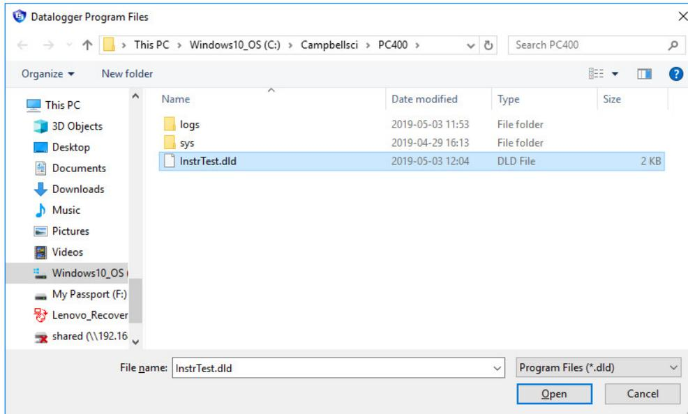
In this example, the program is called 'InstrTest.dld'. The extension 'dld' indicates a program file containing a program that can be sent to a logger.
