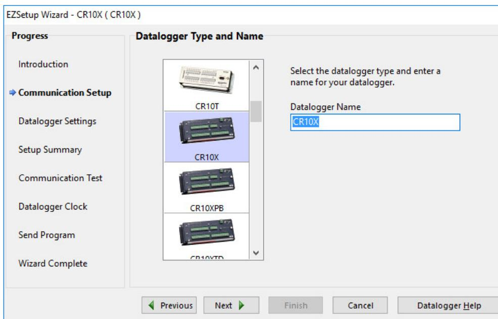
In this example I have chosen the CR10X logger and highlighted the default name 'CR10X'. I strongly recommend that you name your stations with a unique and understandable name. This will help you tremendously if you have many logger stations running in different places or running different tasks since everything associated to that station will be identifiable by the name. Once we have named the logger we can continue by pressing 'Next'.
