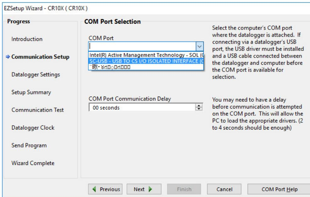
If you have installed the driver for the SC-USB interface and have connected the computer to a logger using this interface you should obtain one option looking like the example above. The SC-USB interface and its driver makes the computer believe one of the USB ports is a serial port, which is what is needed for the interface. Chose the SC-USB option and continue with 'Next'
