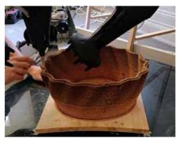
Figures 10-11. Adjustments During Printing. While printing a large scale object, different resistances emerged that required rapid reflection and action from the designers. An example of a resistance encountered here was the warping of the wooden print surface as it absorbed moisture from the print material. The artefact's circular foot-
