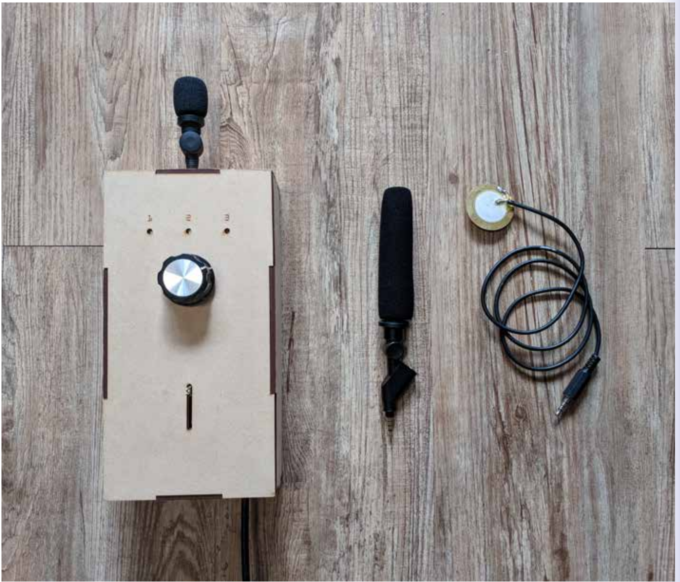
Figure 7. Flâneur's Phonograph with 3 types of microphone: 1) Omnidirectional, 2) hypercardioid, 3) contact mic (from left to right)
